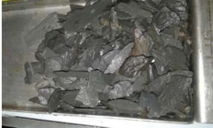
Fig 06: Cavings found in Mubarakpur-1 with in depth 3505-3530m.
