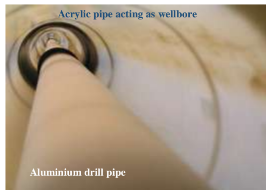
Figure 1: Inside of the 85' long test section (Sagheer, 2009)
