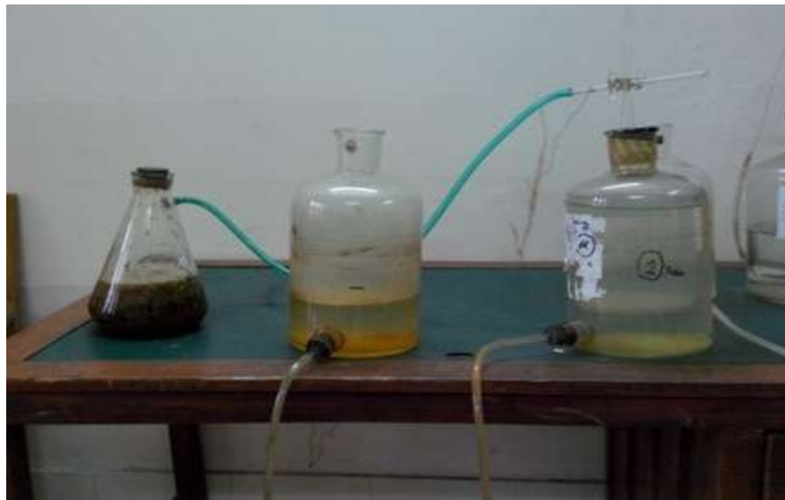
Figure 3. Experimental set-up of a producing biogas from maize stover
