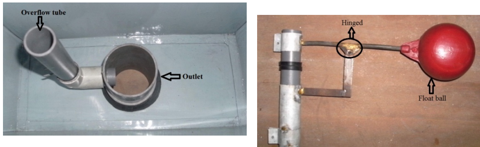
Figure 3: Photograph of the fabricated cistern parts: inside the cistern (left); hinged assembly (right).
