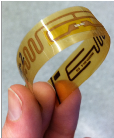
Fig.10. A fully functional flexible electronic device (an RFID tag) fabricated using the LEAP technology.
