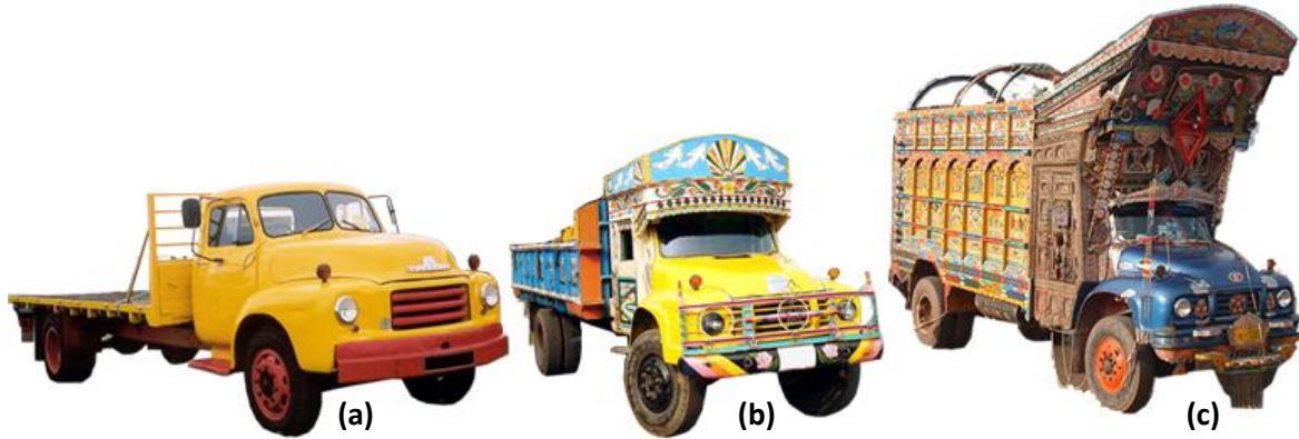
FIGURE 1. Full scale trucks: (a) A Bedford J series truck model without any modification, (b) Modified truck (Bangladeshi), (c) Modified truck (Pakistani).
