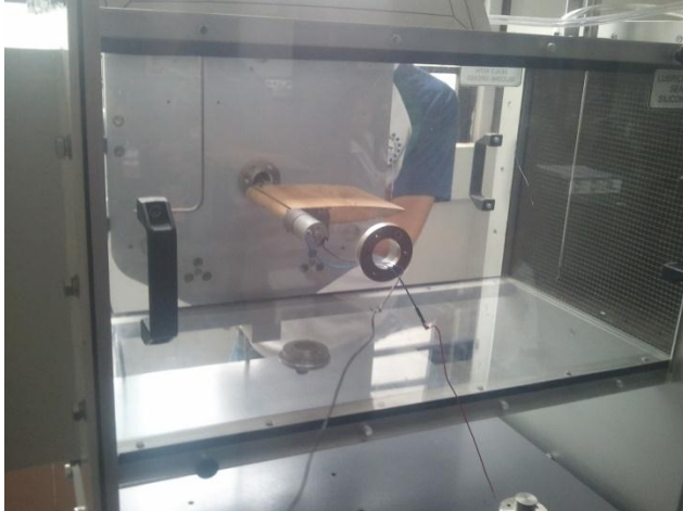
FIGURE 6. Modified NACA 0010 airfoil with cylinder
