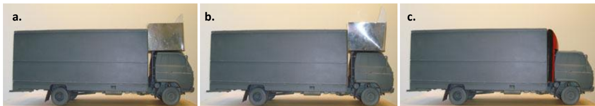
FIGURE 2. Baseline truck fitted with deflector: (a) Bangladeshi, (b) Pakistani, and (c) Aerodynamic.
