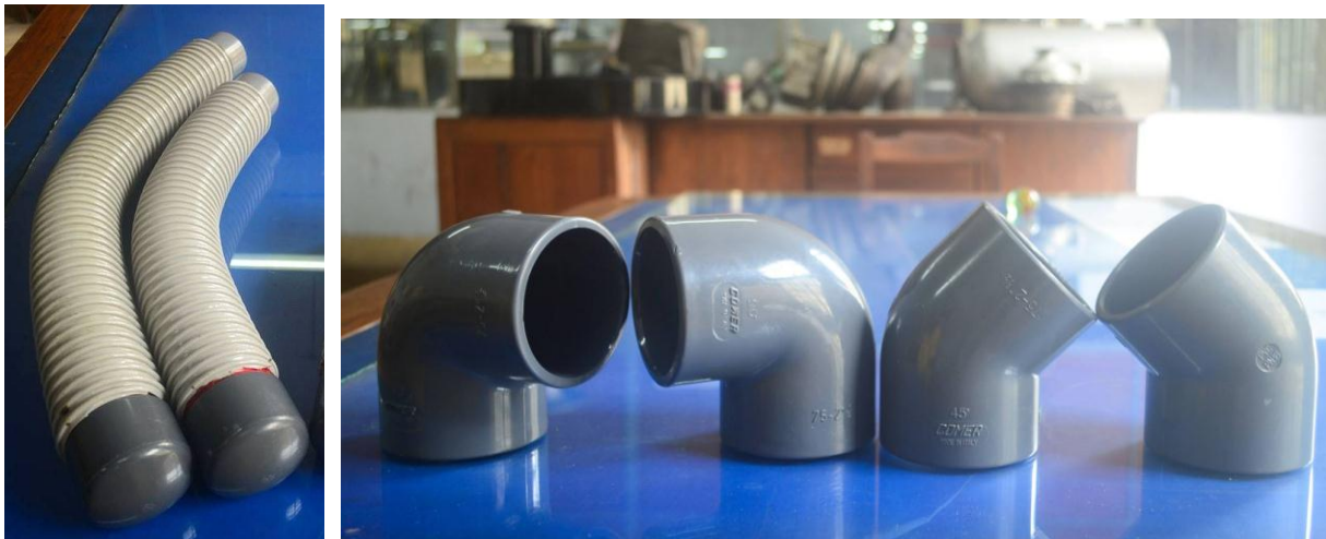
FIGURE 2. Replacing straight PVC tubes with corrugated ones and use of bends to reduce space occupied.
