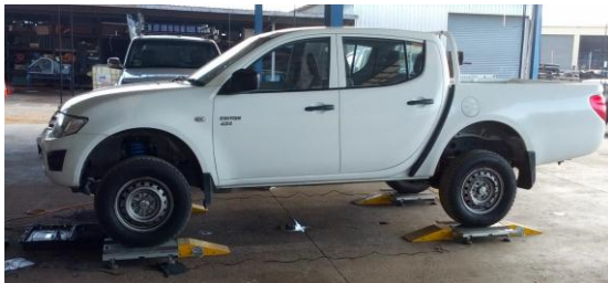
FIGURE 1. Determination of mass distribution of the sample vehicle (Mitsubishi Triton)
