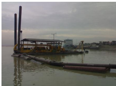
FIGURE 1. Hydrotransport pipeline of a river dredging system (left) and an eroded impeller of its pump (right).
