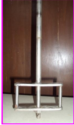
FIGURE 3. The specimen holder attached to the spindle.
