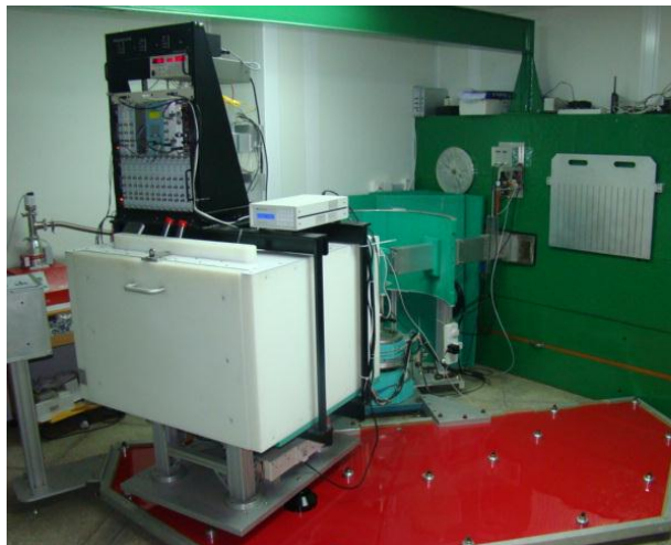
FIGURE 5. The complete setup of the SAND at the reactor beam port.
