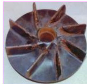
FIGURE 1. Hydrotransport pipeline of a river dredging system (left) and an eroded impeller of its pump (right).
