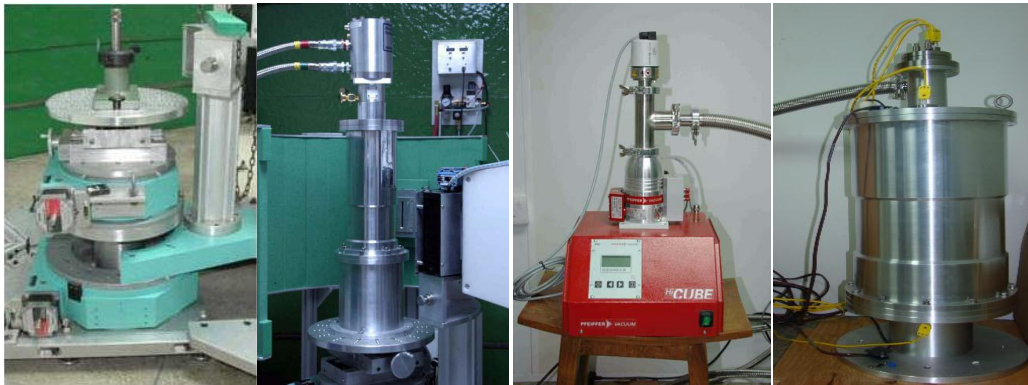
FIGURE 4.(a) Huber sample table (b) Cryo refrigerator (c) Vacuum pump (d) High temp. furnace
