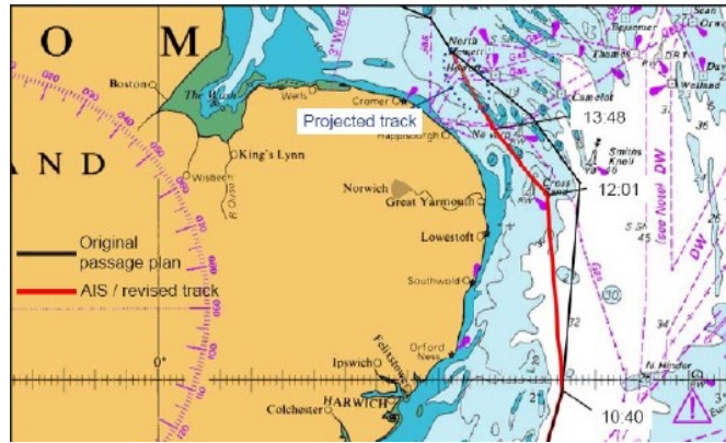
FIGURE 1: Vessels original and revised planned routes. Source: (Report on the investigation of the grounding of CFL Performer, 2008)
