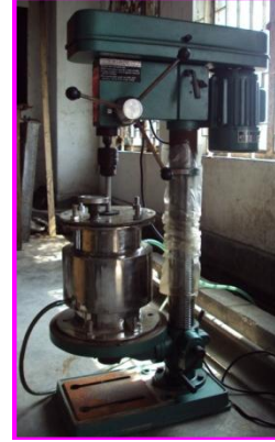
FIGURE 4. The slurry pot tester with the spindle attached a drilling machine.
