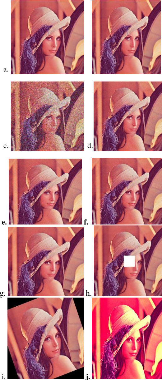
Fig. 5: Pictorial representation of watermarked image under different attacks (a) Original host image, (b) watermarked image, (c) Gaussian noise (0.1), (d) Speckle noise (0.01), (e) Salt & pepper noise (0.01), (f) Poisson noise, (g) JPEG Compression (q.f=60), (h) Cropping 80x80, (i) Rotation 20°, (j) Contrast adjustment
