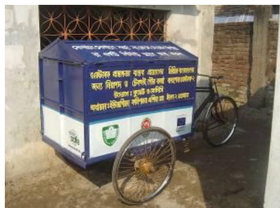
Figure 4: (a): Existing waste collection rickshaw Van (b) Newly designed waste collection
