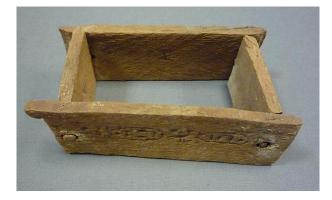
Fig.3 Hand made brick mold
