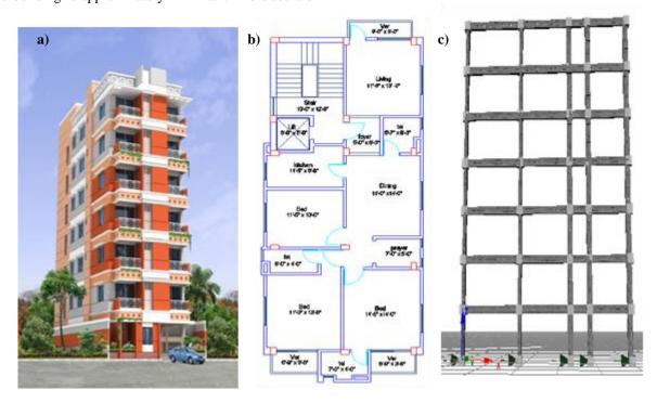
Fig.1 The studied structure: a) Full scale building, b) building layout, c) finite element model
