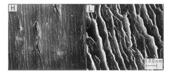
**Fig. 5** Fractographs of specimens after fatigue crack propagation test for 2024 aluminum alloys with wide (H) and narrow (L) spacing of dispersoids. [5]
