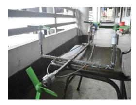
Fig. 2 Construction of UAV body.
