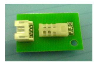
Fig.5 HSM-20G humidity sensor
