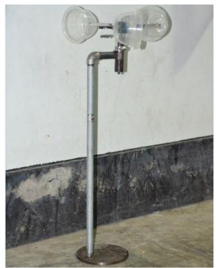
Fig.3.1 Constructed Anemometer
