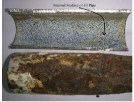
Fig.2: The sample GI pipe used for carrying sample water
