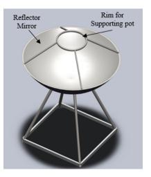
Fig.3 Parabolic solar collector
