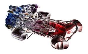
Fig.1 The Rolls-Royce Pegasus V/STOL Engine
