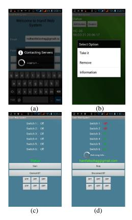
**Fig.8** Screen shots of some processes, (a) Logging to the server, (b) Connecting to Bluetooth Module (HC-05), (c) Devices status, (d) Receiving information from the server.
