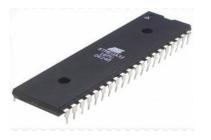
Fig.13 ATMEGA 32 microcontroller
