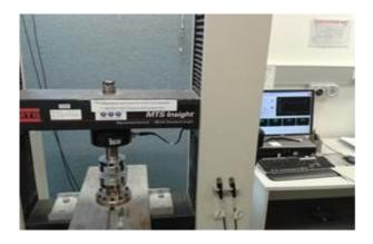
Fig.4 MTS Insight machine for compression testing
