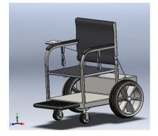
Fig.3 Isometric view of designed wheelchair
