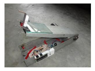
Fig.2 A Digital Sliding Friction Tester after construction.
