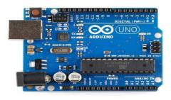
Figure 2.4: Arduino Board (UNO)
