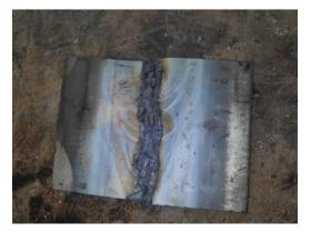
Fig. 6: A butt welded workpiece
