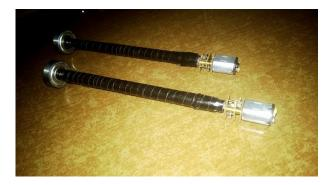
Fig.3 Gear Motor, Shaft and Bearing arrangement
