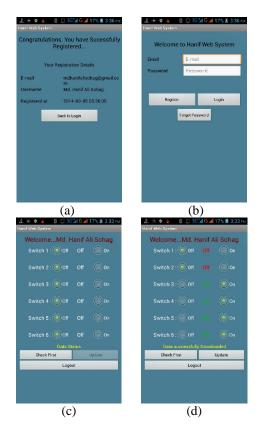
Fig.9 Screen shots of some processes, (a) Registering to the server, (b) Logging to the server, (c) Devices status, (d) Devices status changed.
