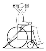
Fig.8 A typical wheelchair tie down and occupant restraint system (WTORS).
