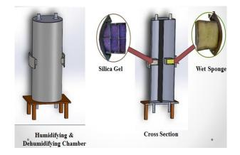
Fig.3 Humidifying and dehumidifying chamber
