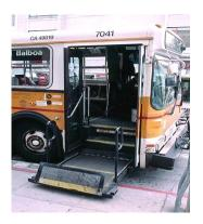
Fig.1 A wheelchair lift in the front door of a low floor city bus in San Francisco
