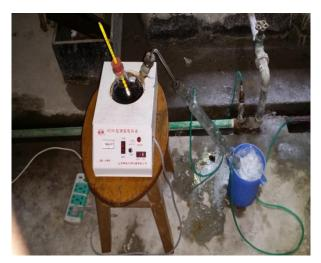
Fig.2 Thermal cracking apparatus
