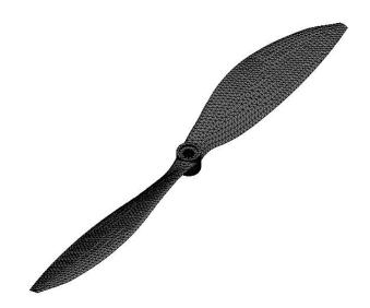
Fig.7 3D meshing over the surface of propeller blades
