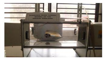
Fig.2 Experimenting the modified wing in wind tunnel.
