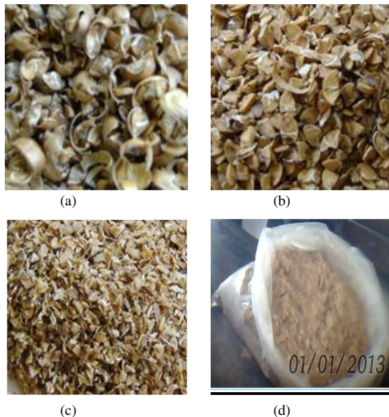
Fig.2 (a) Crushing, (b) Seed bark separation, (c) Final crushing and (d) Powder production.
