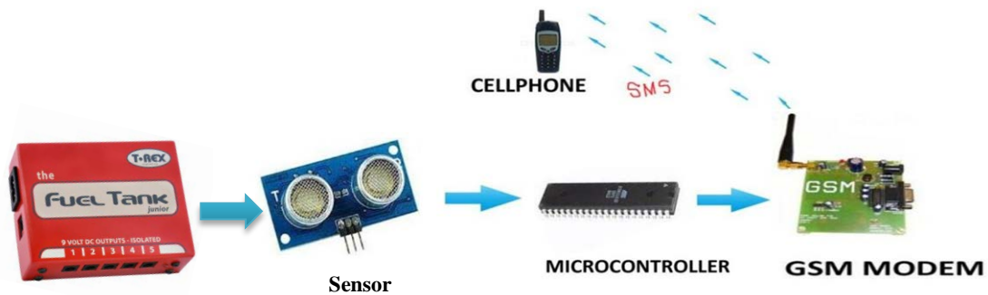
Fig. 3. Overall system design for drastically fuel loss of the vehicle.
