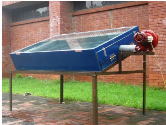
Fig.3. Experimental set up of solar air heater
