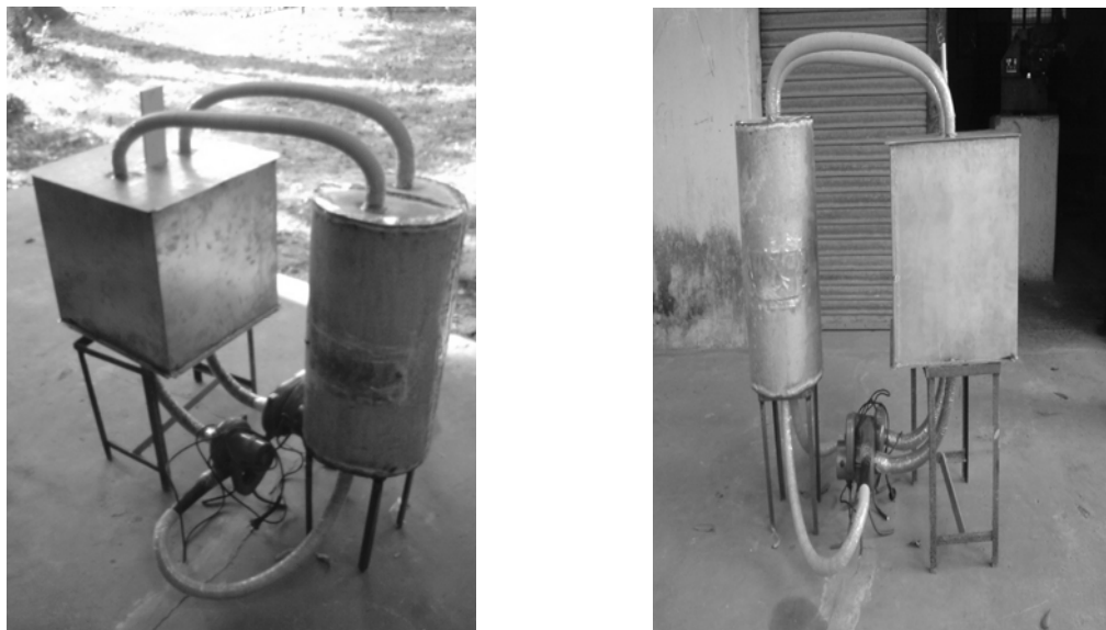
Fig. 8. Photograph of the complete assembly of humidity control system
