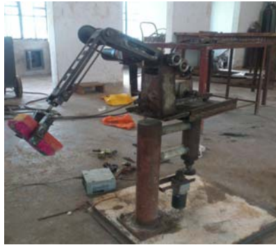
Fig. 6. Robotic arm lifting objects of average
