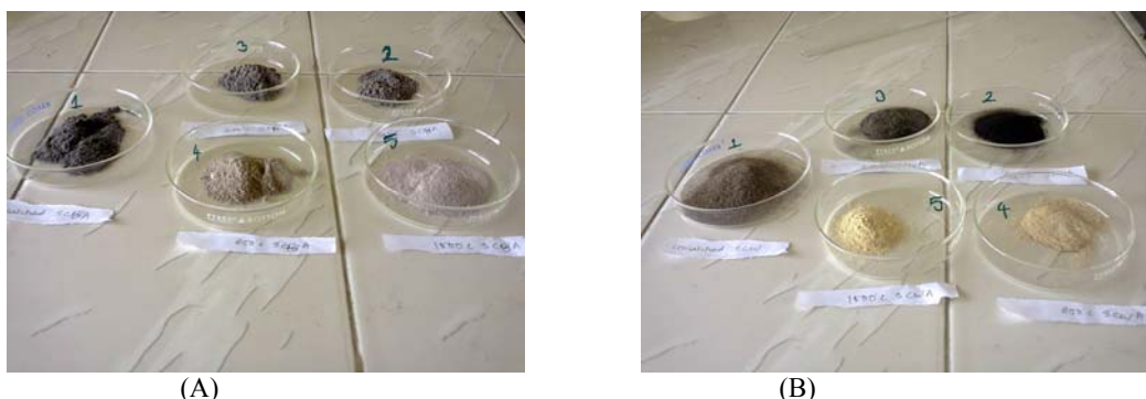
Figure1. (1)Uncalcined bagasse ash (A) and Sugarcane waste (B) and calcined at different temperature (2) 400°C (3) 600°C (4)800°C and (5) 1000°C
