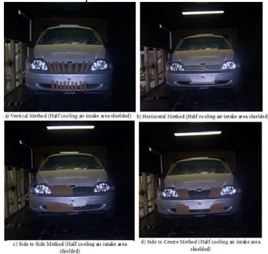
Fig. 5. Test vehicle at RMIT Industrial Wind Tunnel [7, 29]
