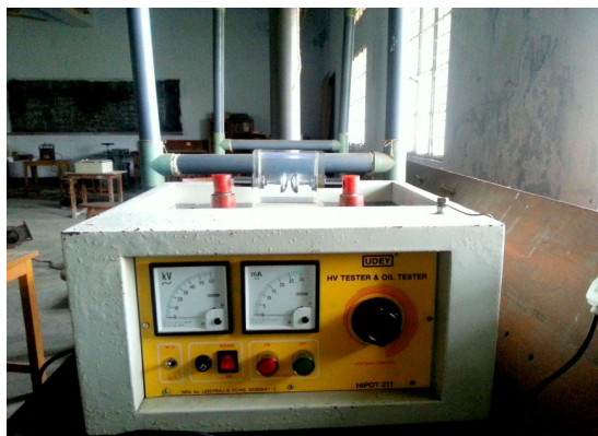
Figure1. Liquid dielectric test set, model OTS-E Series for breakdown voltage measurement.
