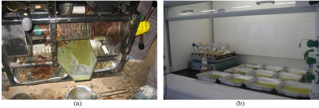
Figure 5: (a) Mechanical oil extraction through a screw press (b) Chemical oil extraction
