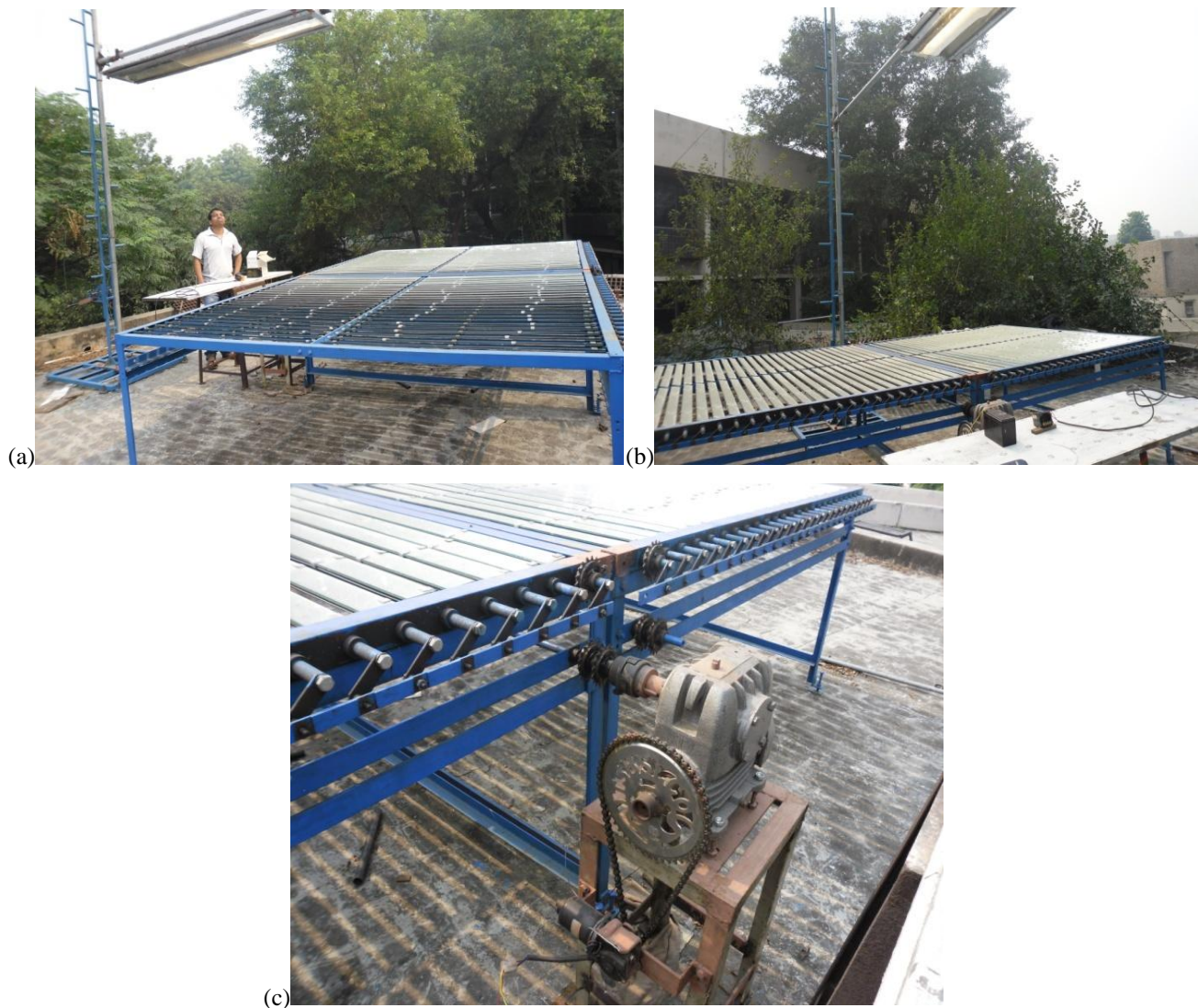
Fig. 6. (a) fresnel concentrator setup, (b) another view of setup with tracking timer, (c) Tracking motor with gear box and linkage mechanism
