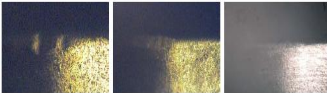
Fig. 5: (a) tool wear in cutting normal work piece without magnet, (b) tool wear in cutting normal work piece with magnet, (c) tool wear in cutting heat treated work piece with magnet
