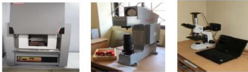
Fig. 2: (a) Heat treatment furnace, (b) Rockwell hardness testing machine, (c) Optical metallurgical microscope set up
