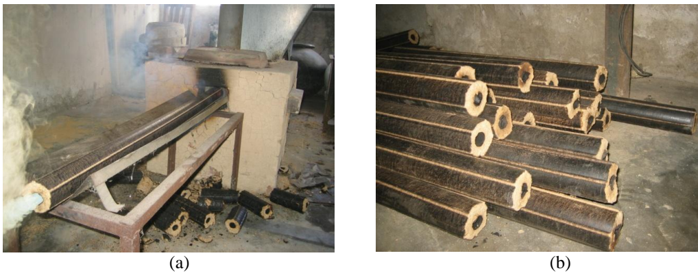
Figure 5. (a) Showing briquette coming out from brick-clay die stove and (b) the briquette
