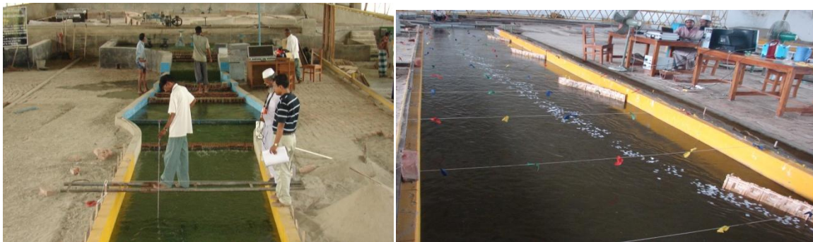
Fig.1: Experimental set-up for the open channel with the water supply system
