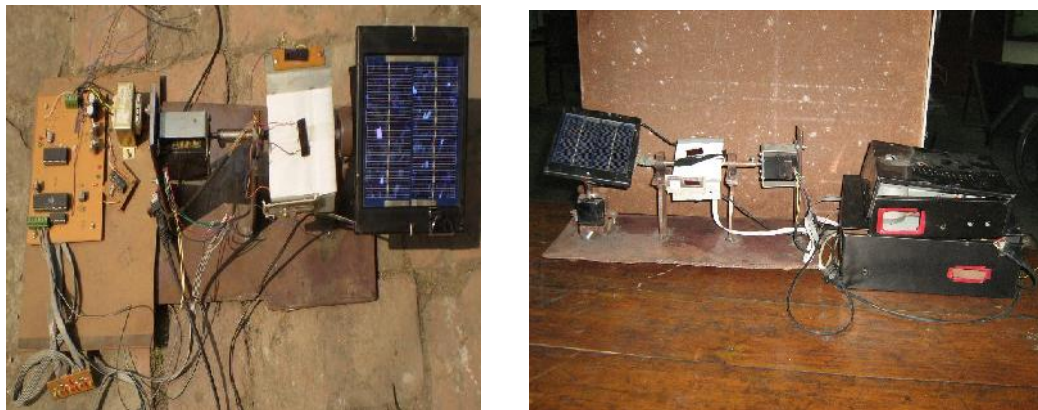
Fig. 4. Experimental set-up of (a) single axis tracker; (b) Two axis tracker
