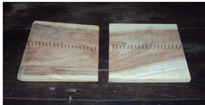
Fig. 2. Airfoil NACA 0015, Flat Plate Model
