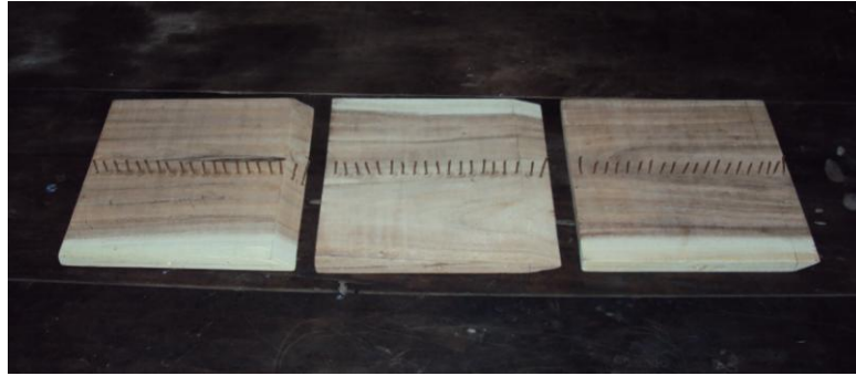
Fig. 4. Modified Flat plates with modified after-face (MFP4, MFP5, MFP6)
