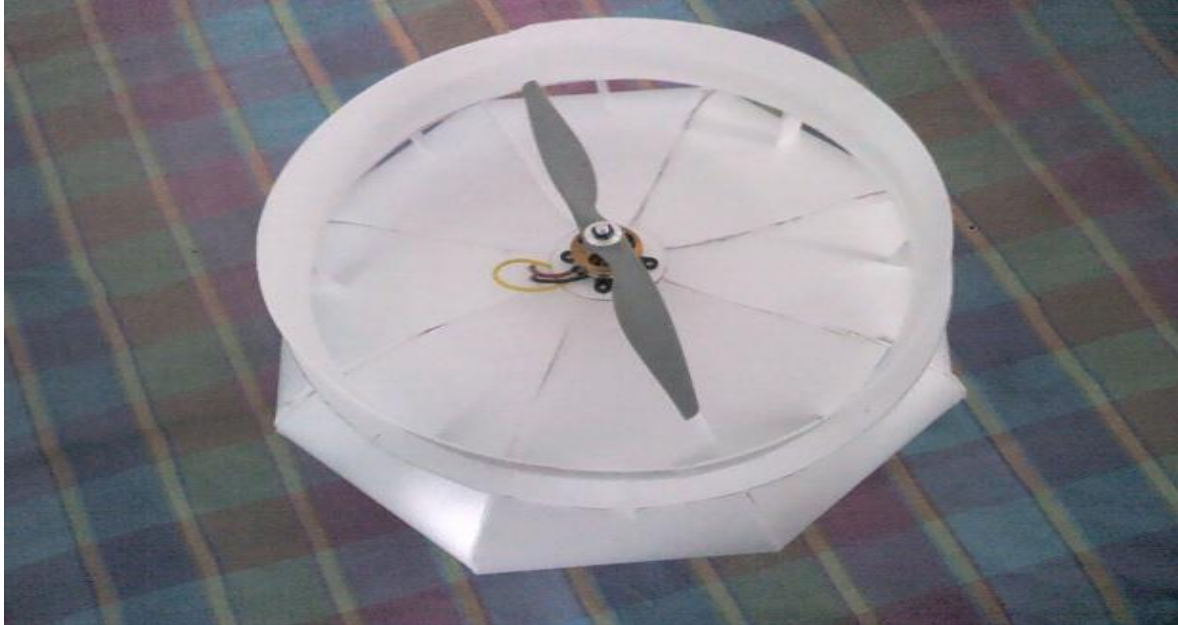
Fig 13. Final structure of the UAV(Coanda effect flying saucer)
