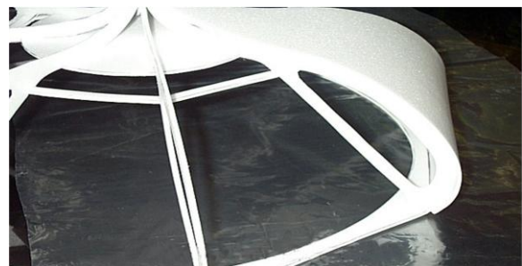
Fig 12. Attachment of the curved petal parts to the main frame
