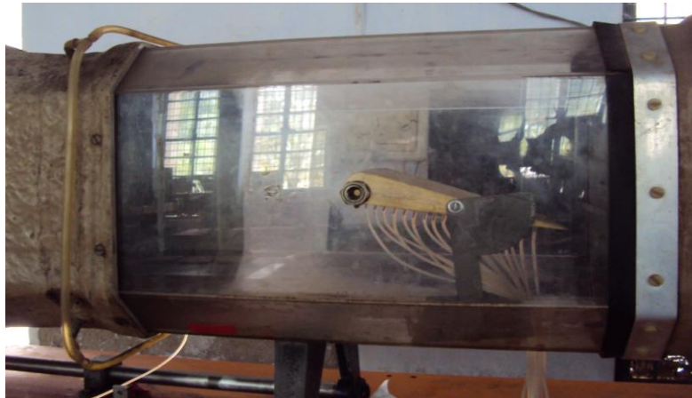
Fig. 5. Experimental setup( The NACA0015 airfoil mounted in the wind tunnel)
