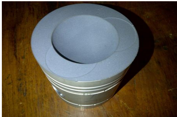
Fig.1. AV1 Diesel engine piston coated with Titanium dioxide
