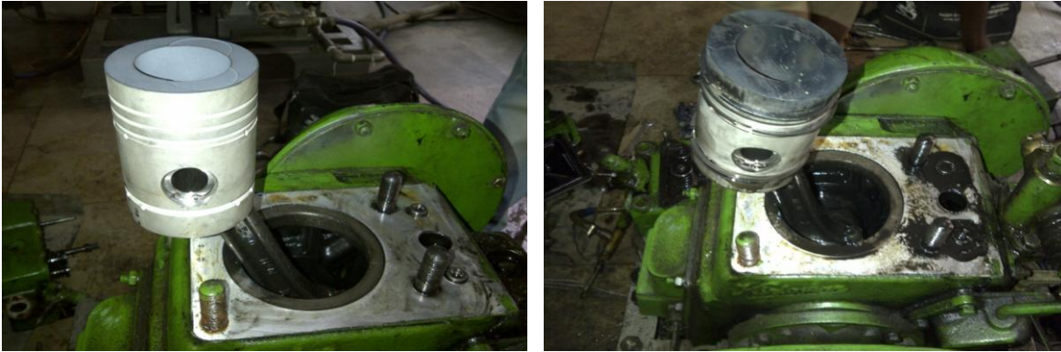
Fig. 2. (a) Coated piston before engine is run (b) Coated piston after engine is run.
