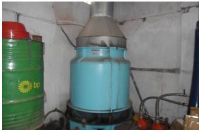
Fig. 7 Condenser is used to cool down plastic goods
