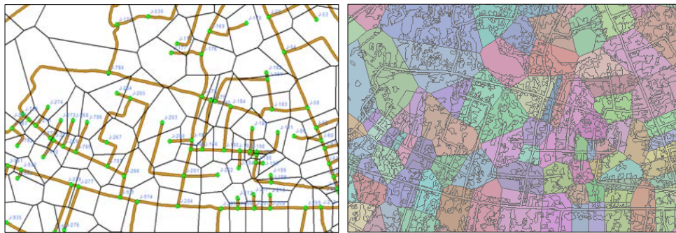
Fig. 2: (a) Nodal area demarcation using Thiessen Polygon and (b) Union of shape files for nodal water demand computation database.
