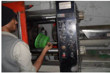
Fig. 8 The product has been molded and taken out
