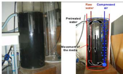
Figure 3: Meteor Pilot Unit & Flow Diagram.
