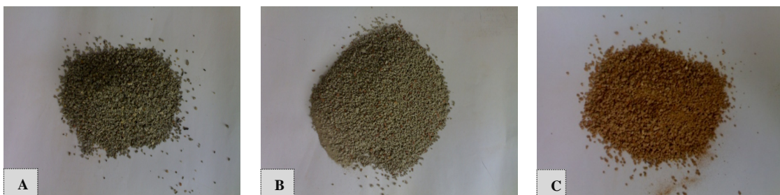
Fig. 1. Sample of prepared fine aggregate from A) brick aggregate concrete B) stone aggregate concrete and C) lime aggregate concrete
