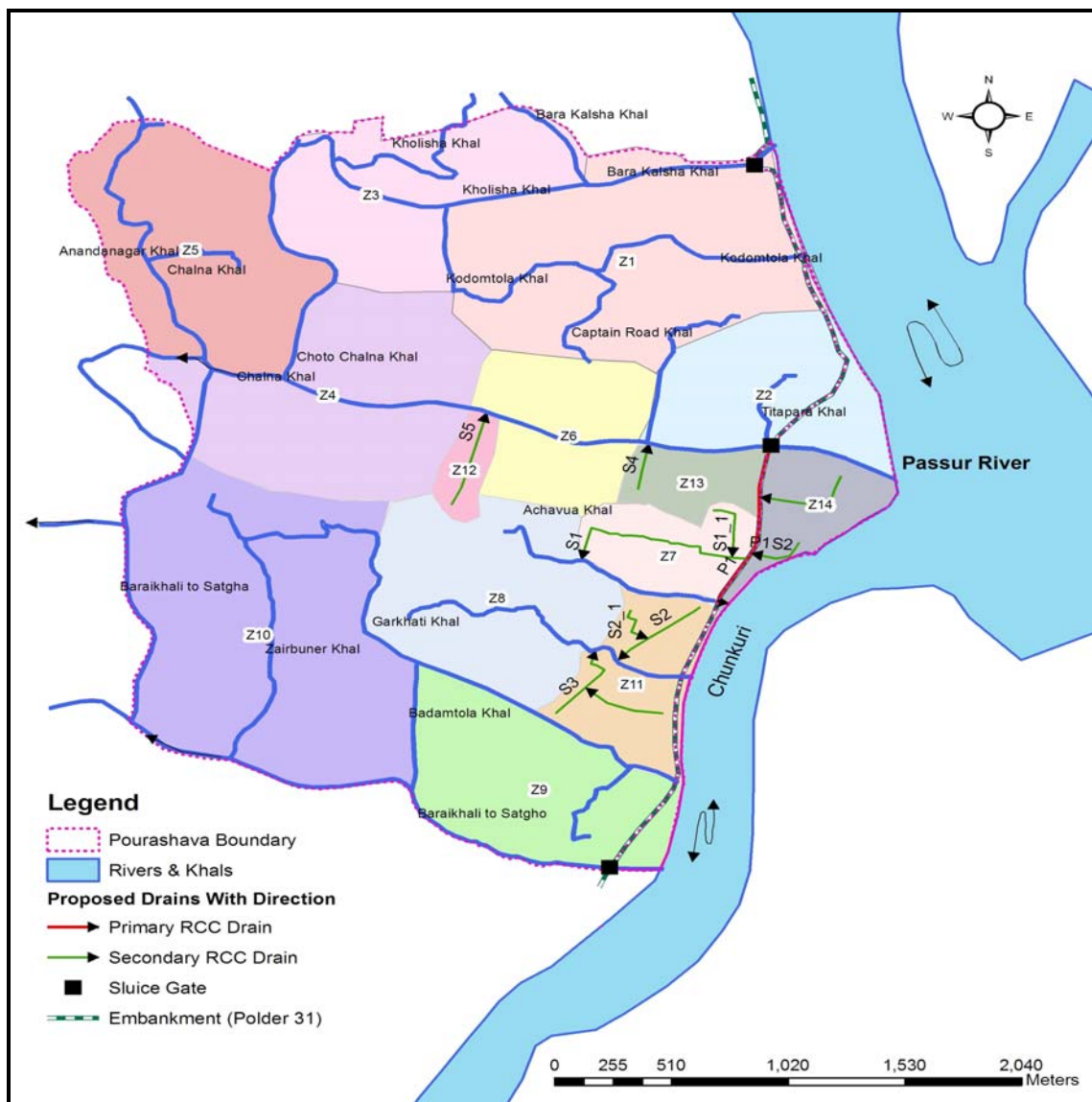
Fig 1: Drainage Zones and proposed drains with outfall
