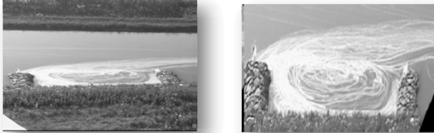
Figure 3 : Example of flow behavior in open channel flow with rectangular side cavity (Muto et al., 2002)
