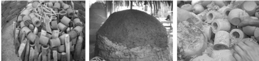
Figure 7: Filter burning in Potter kiln
