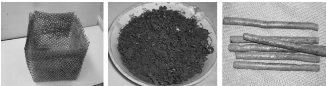
Figure 9: Iron net, scrap iron and iron rod for the filter unit
