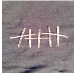
Figure 4: PET fibers produced from bottle
