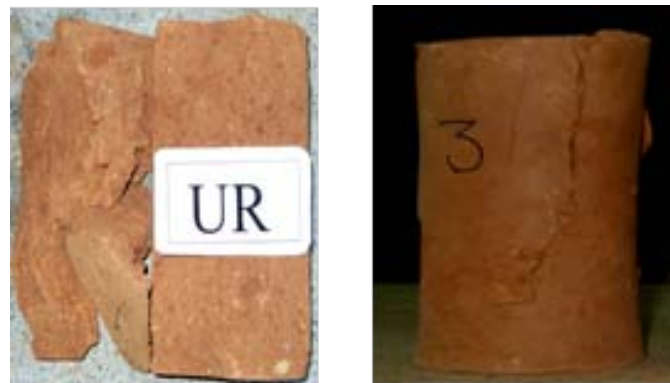
Figure 4: Failure pattern of unreinforced (left) and jute reinforced block (right)
