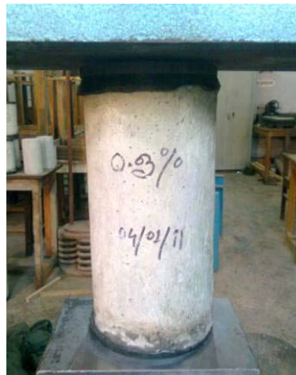
Figure 10: Instrumentation of cylinder specimen to test the compressive strength
