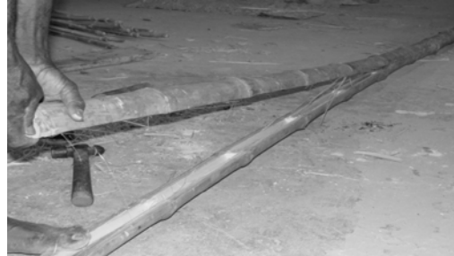
Figure 2: Bamboo splitting into two pieces
