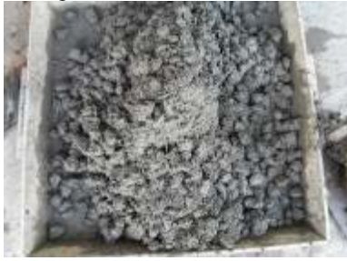
Figure 8: Concrete with PET- Fiber
