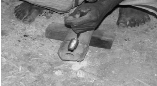
Figure 1: Hammering bamboo with a chisel
