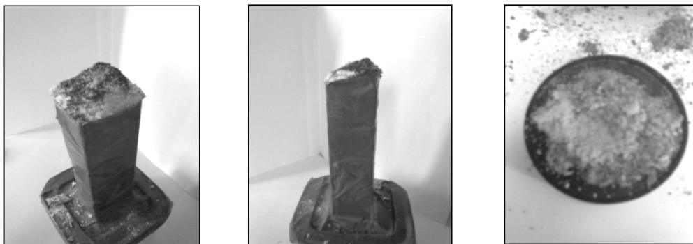
Figure-10: Distressed brick top due to One directional Flow of Distilled Water
