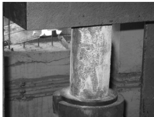
Figure 4: Typical setup for compressive strength test
