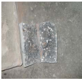
Figure 18: Brittle failure of specimen T_1
