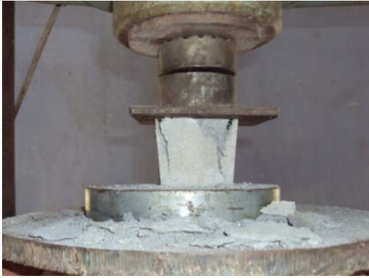
Figure 3: (a) Compressive strength experimental set up (b) Bond strength experimental set up
