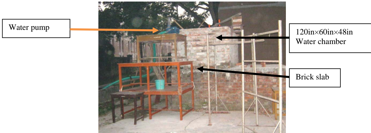
Figure 7: Application of water pressure on masonry slab.
