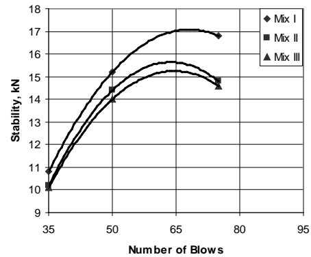
Figure 5: Relation between density and No. of blows Figure 6: Relation between stability and No. of blows
