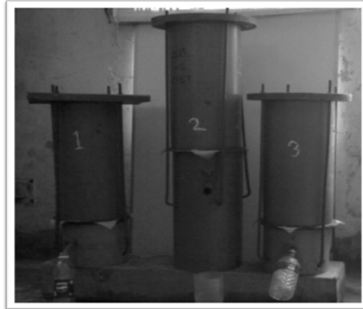
Figure 2: Three laboratory test setups of clay liner system
