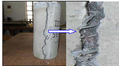
Figure 19: Fiber bridging of specimens T_2 , T_3 and T_4
