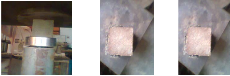
Figure 2: Failure load taken by Universal Testing Machine
