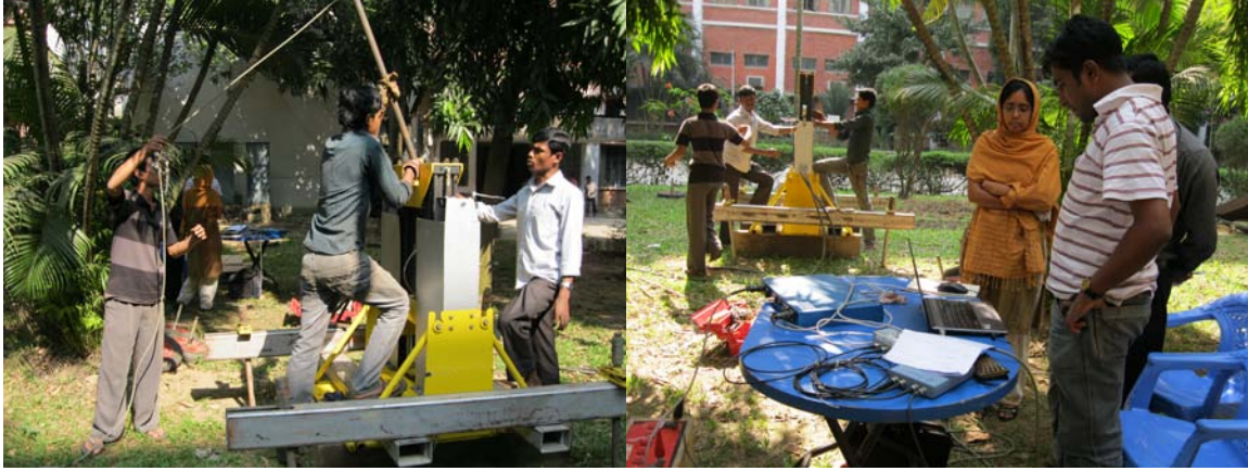
Figure 3: Cone Penetration Test demonstration at BUET campus.
