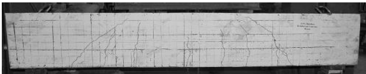
Figure 22: Failure pattern for 2.5% bamboo reinforced beam.
