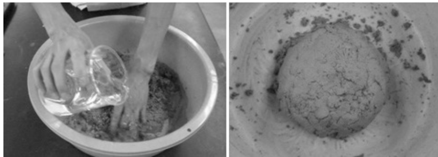
Figure 3: Mixing of soil and rice bran and making of dough with water
