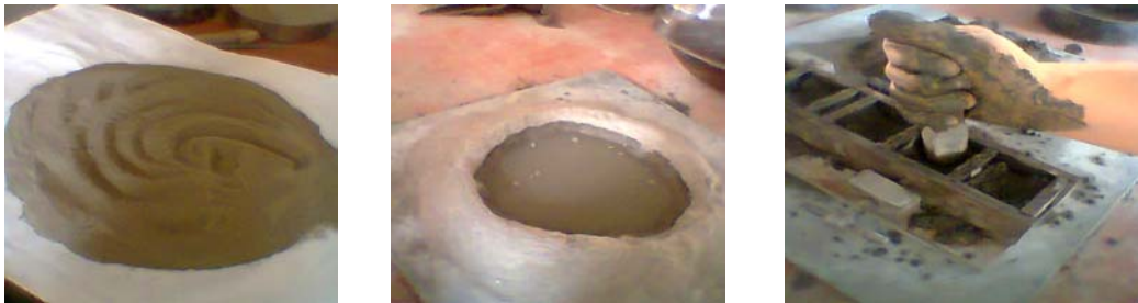
Figure 1: Preparation of cement mortar
