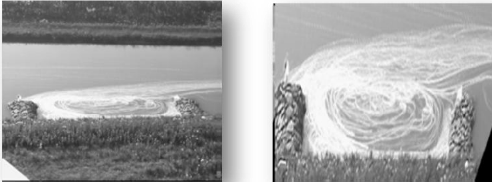
Figure 1 : An example of flow behavior in rectangular side cavity (Muto et al., 2002)
