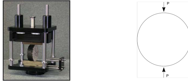
Figure 2: (a) Indirect Tensile Strength test setup, (b) Simplified 2D diametrically point loaded disk
