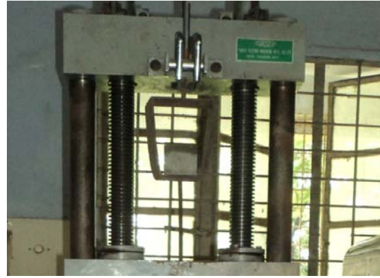
Figure 3: (a) Compressive strength experimental set up (b) Bond strength experimental set up
