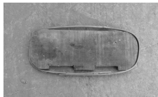
Figure 9: Water soaked split bamboo was wound around the wooden form
