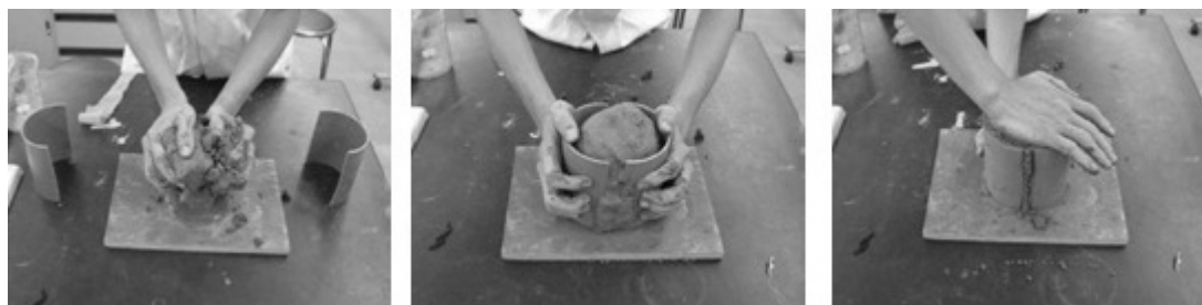
Figure 4: Shaping of filter from dough using dice
