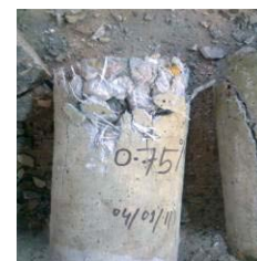
Figure 16: De-bonding of fiber-matrix of specimen C 4
