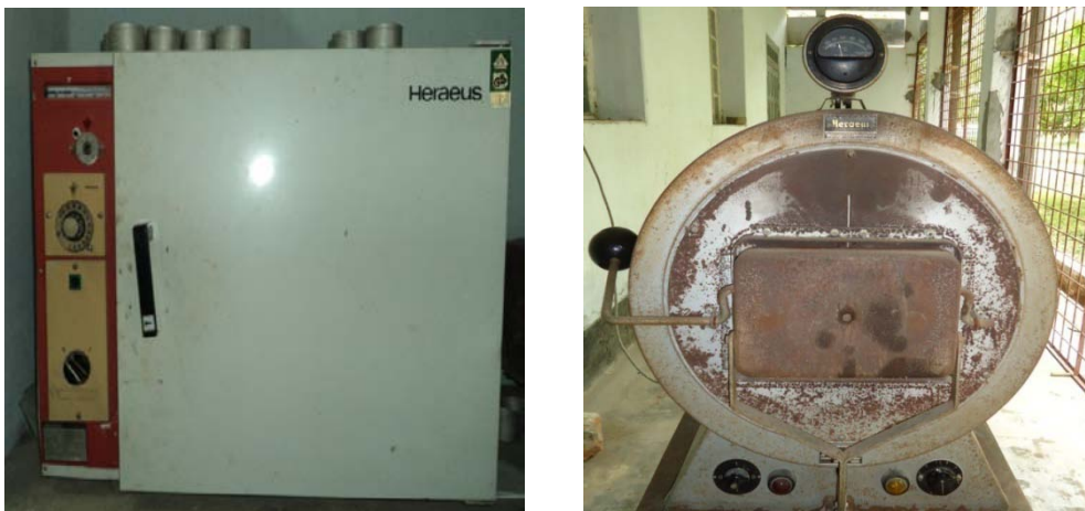
Figure 2: Heating arrangement (a) electric oven (b) electric furnace
