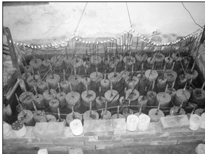
Figure 4: Parallel connection in corrosion cell
