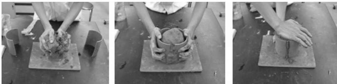
Figure 4: Shaping of filter from dough using dice
