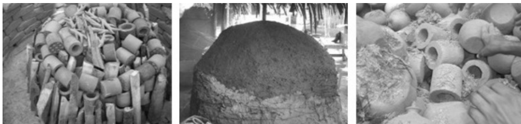
Figure 7: Filter burning in Potter kiln
