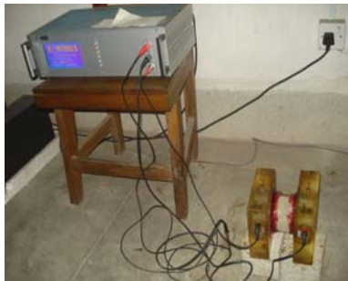
Fig 7: Test Arrangement for RCPT
