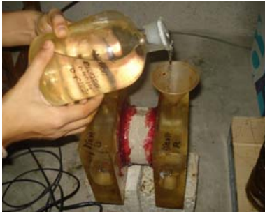
Fig 4: Pouring 0.3% NaOH Solution in Other Cell
