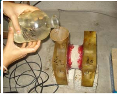
Fig 3: Pouring 3% NaCl Solution in One Cell
