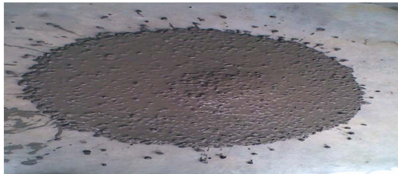
Fig 2. Free Flow Concrete
