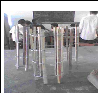
Figure 03: Preparation of bamboo reinforcement case with tie bar.
