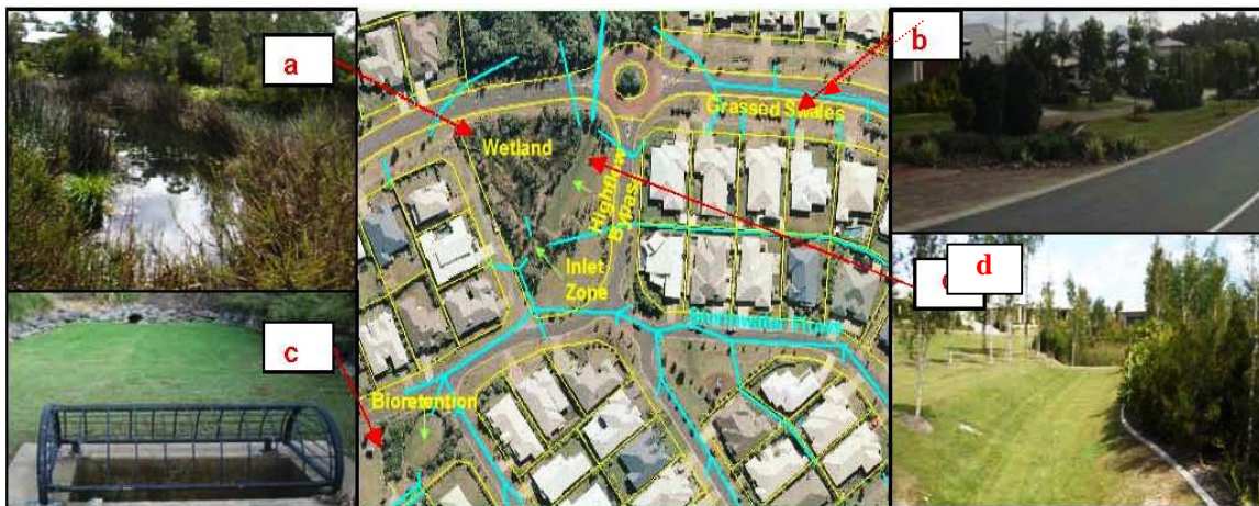
Figure 8: WSUD elements in Coomera Waters; a. Wetland Macrophyte Zone, b. Swales & driveways, c. Bioretention d. High flow bypass of wetland (looking upstream).
