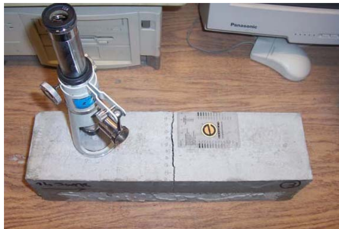
Figure 5: Crack Measurement Using a Microscope
