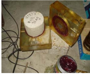
Fig 2: Sealing of the Sample with the cell
