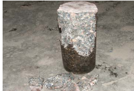
Fig-5 (b): Polymer concrete after failure
