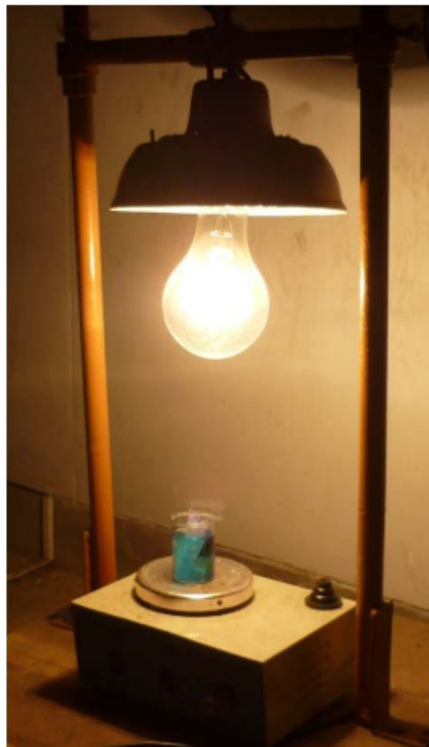
Fig 1. photo degradation of methylene blue under visible light irradiation.
