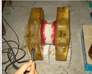
Fig 5: Attaching Connector with Cell Containing 3% NaCl Solution
