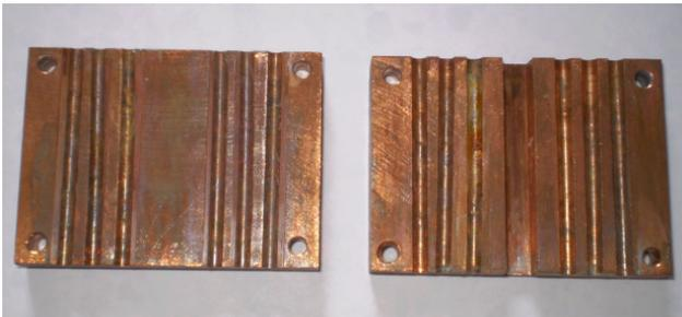
Fig. 2 Grooves cut in the copper blocks for inserting MHPs evaporator section.
