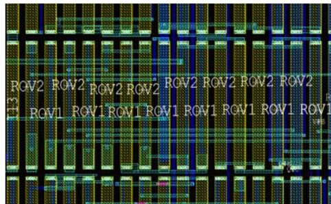
Fig. 3 Inter-digitization of resistance divider in layout to reduce offset in the circuit
