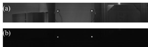
**Fig. 4 Examples of the image windowed with 752  $\times$  102 pixels captured by the prototype system: (a) normal image and (b) IR image through the IR-pass filter.**
