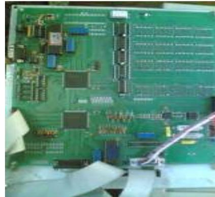
Fig. 14. Micro-controller mounted on the back of the keyboard.
