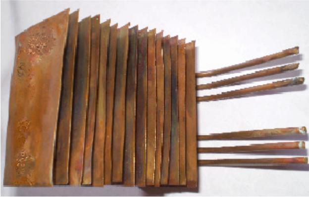
Fig. 1 Extended fins of copper sheet in the condenser section.
