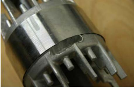
Fig. 1: The Faulty rotor of the IM.
