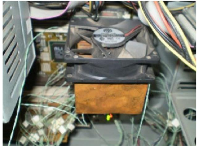
Fig. 6 Experimental setup for cooling desktop by using MHPs with cooling fan.
