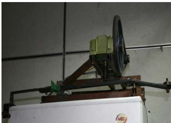
Fig. 1 Automatic door opening mechanism
