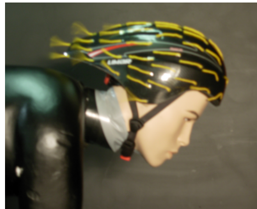
b) Flow visualisation with wool tuft
