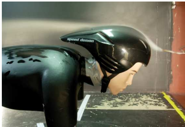
a) Flow visualisation with smoke
