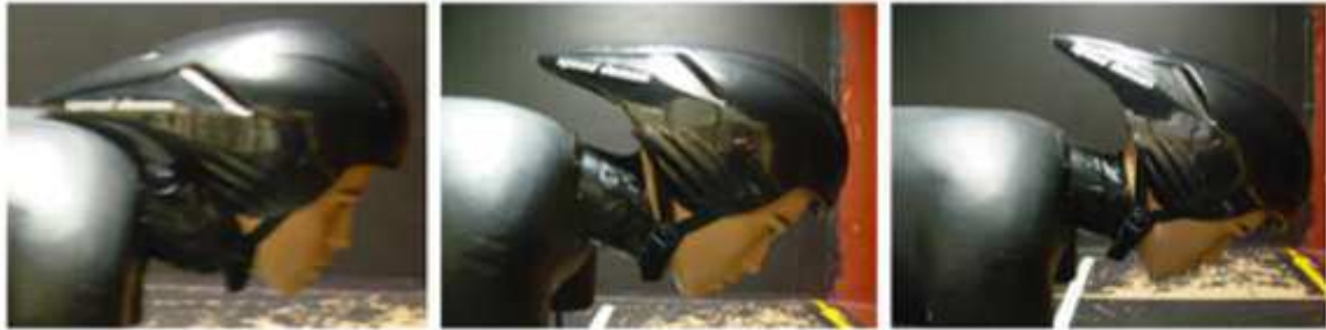
Figure 6: Pitch inclinations used during testing. (Left to Right: 0^\circ [Initial], 15^\circ & 30^\circ )
