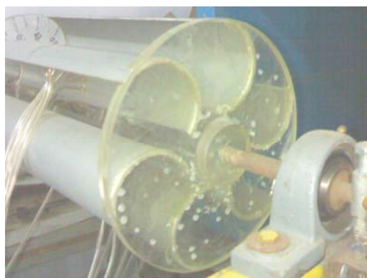
Fig. 2: Six bladed vertical axis vane type rotor.
