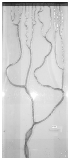
Fig.2 Photographic view of the fluid stream network at a Reynolds number 1900-2000
