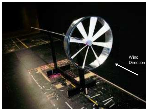
a) Rotating Shroud (Tower Distance 107mm)
