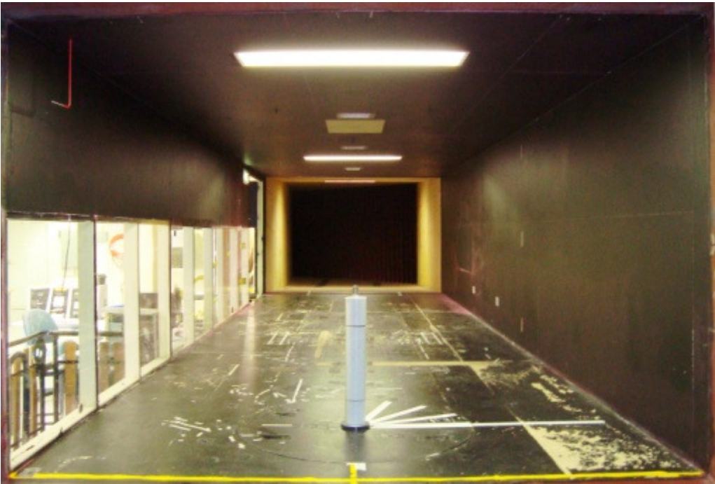
Figure 6: Cylinder with all three sections in the test section of RMIT Wind Tunnel
