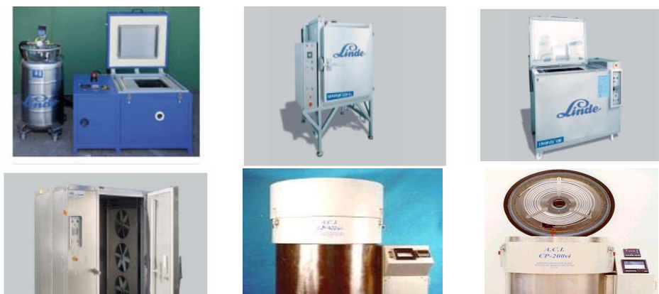
Fig.4 Examples of cryogenic processors by different manufacturers
