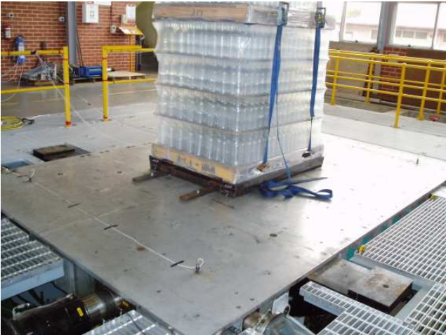
Figure 4: Input Floor with Accelerometers
