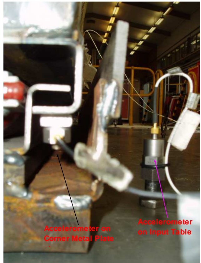
b) Accelerometer on Metal Plate on Air Bag
