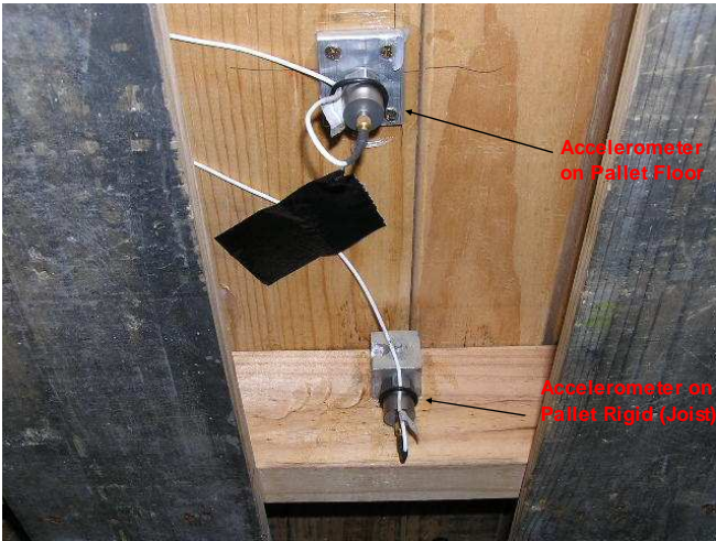
Figure 6: Accelerometers on Wooden Floor above the Metallic Floor on Air Bag
