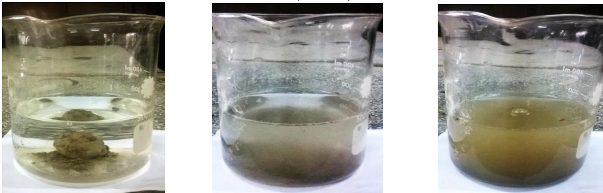
(a) (b) (c) Fig.1: Observation from crumb test: (a) Observation at instant. (b) At 15 minutes. (c) At 1hour
