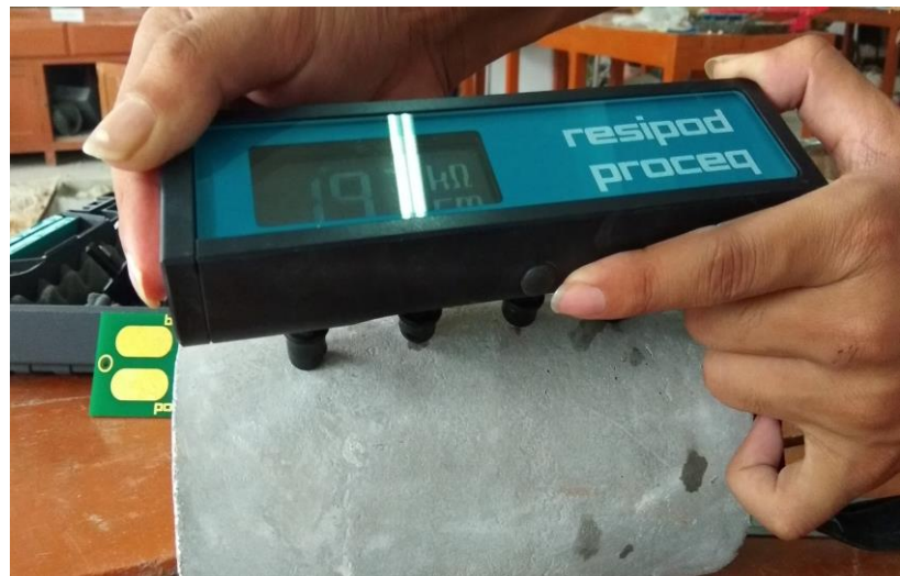
Figure 3: Surface Resistivity test of Concrete cylinder
