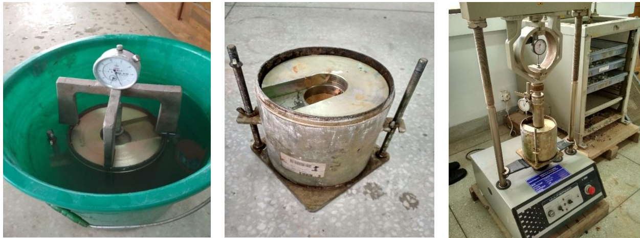
Photo 2 Assembly for finding swelling values and soaked CBR value
