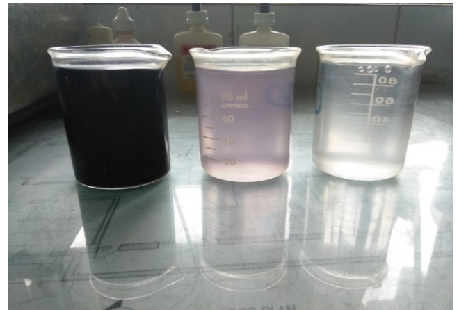
Figure 6: Color variation of wastewater sample of equalization tank, UASB reactor and DHS reactor.
