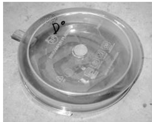
Figure 2: Ignited mosquito coil placed into chamber
