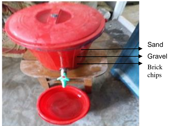
Figure 2: Experimental setup of developed filter
