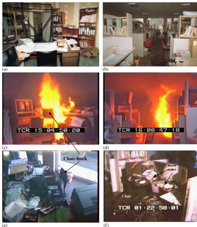
Figure 7. The fire load and size of the fire at the time of sprinkler activation during 140 William St. tests and damage estimate after fire.
