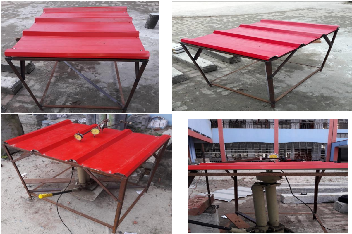
Figure: 12 Test arrangement of wind uplift load
