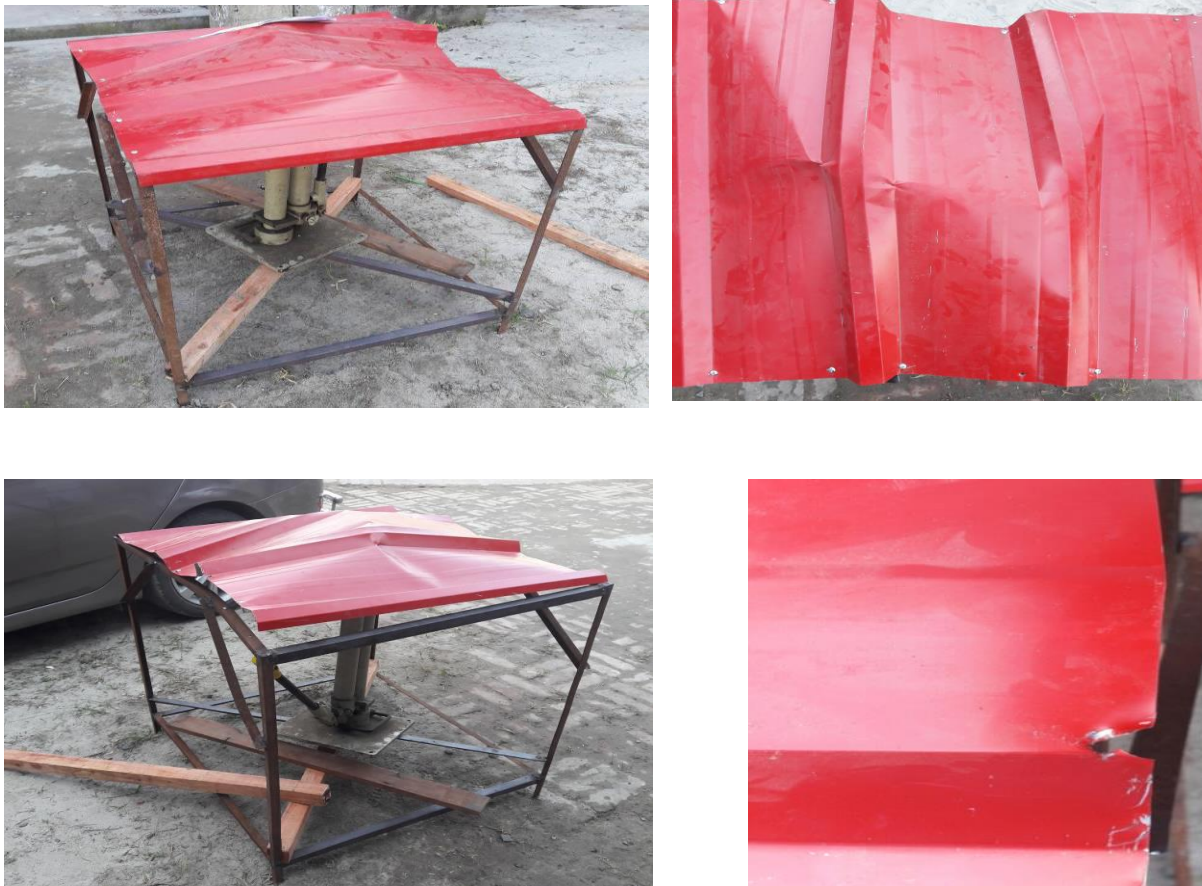
Figure 13: Failure mode of uplift pressure
