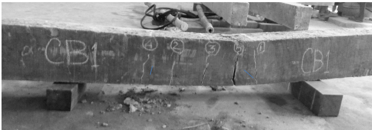
Figure-4: CB-1 after testing
