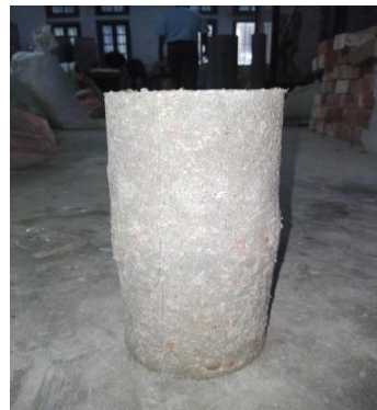
Figure 2: compressive failure at 15% replacement level
