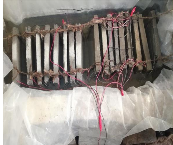
Figure 5: Specimens in Corrosion Cell
