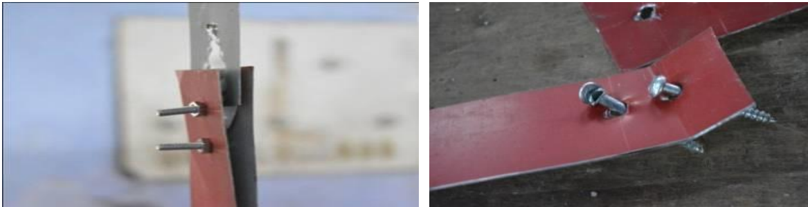
Figure 9: Tested failure mode of screw and bolt connection
