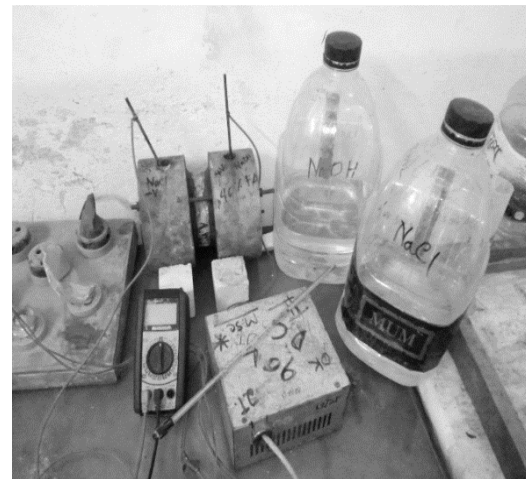
Figure 4: Rapid chloride permeability test setup
