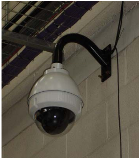
Figure 1: One of 5 web cameras installed in the Bristol laboratory (4 PTZ's and 1 static)
