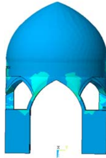
Figure 22. Starting Cracking of the model 2
