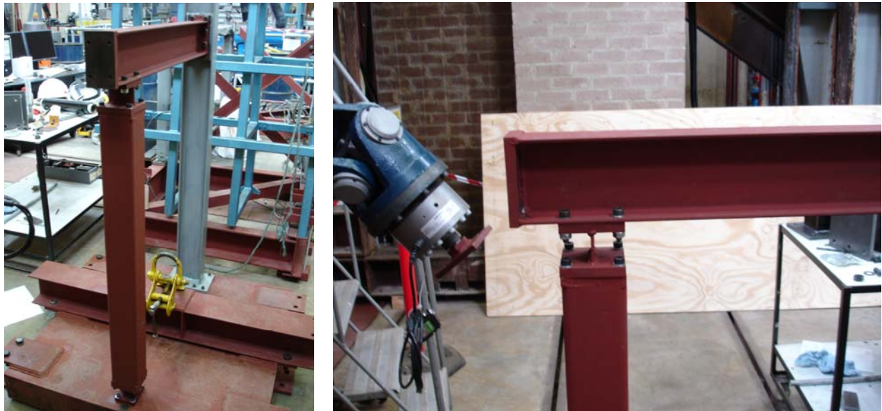
Figure 7: Basic portal frame test (left) and detail of pin connection where actuator is connected (right)
