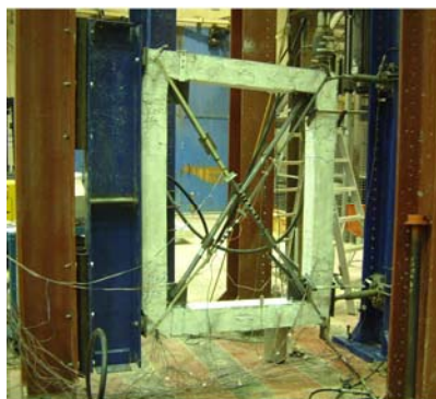
Figure 1. Setup for cyclic testing of specimens
