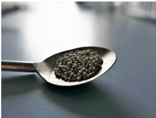
Fig. 7: TiO 2 -coated expanded glass bead granules
