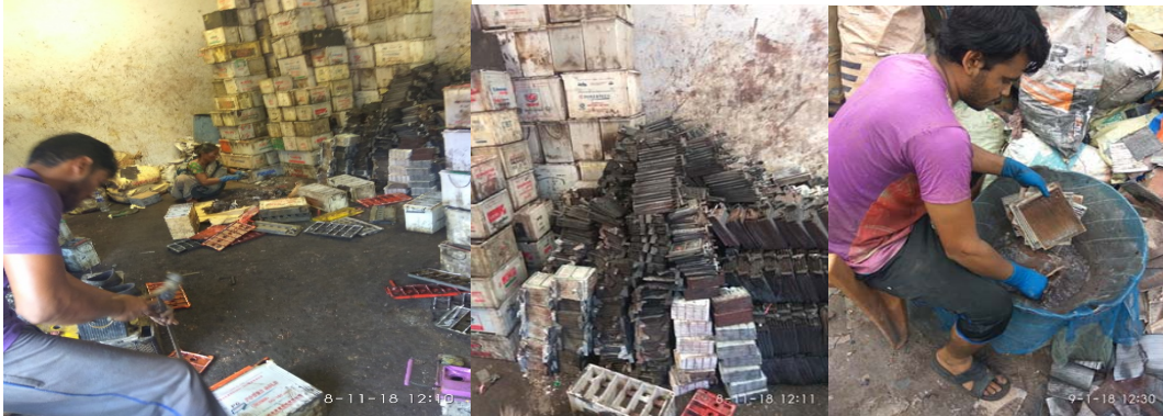
Figure 2 Breaking to Damaged Battery
