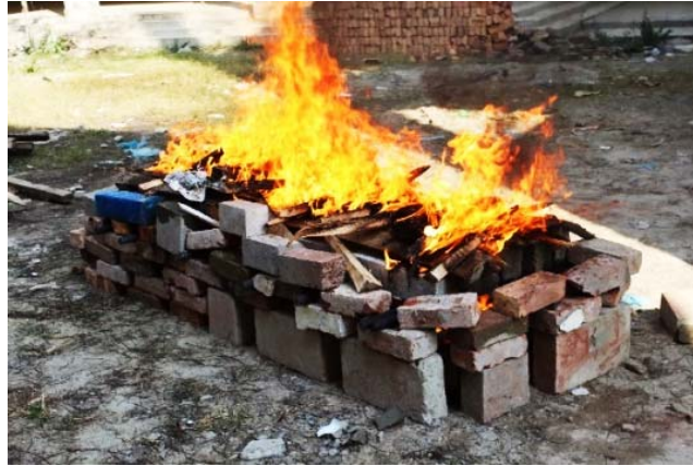
Figure 1 Burning of test specimens in the fire chamber.
