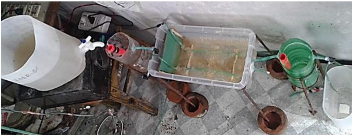
Figure 4: The bench scale biological wastewater treatment plant
