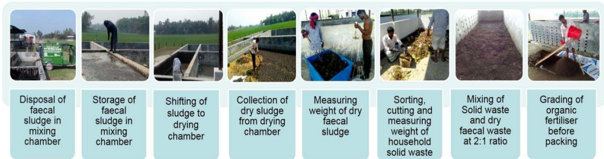
Figure 2: Stages of producing organic fertilizer in the FSM co-composting plant
