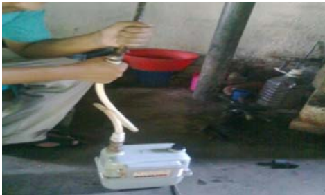
Figure 5: Measurement of biogas using flow meter
