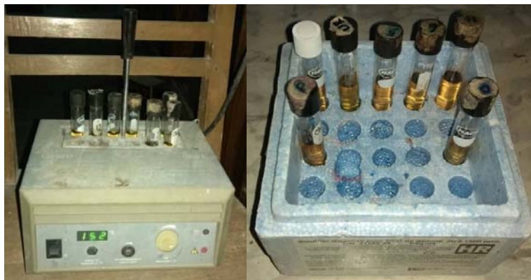
Figure 6 Sample preparation for the calculation of COD.
