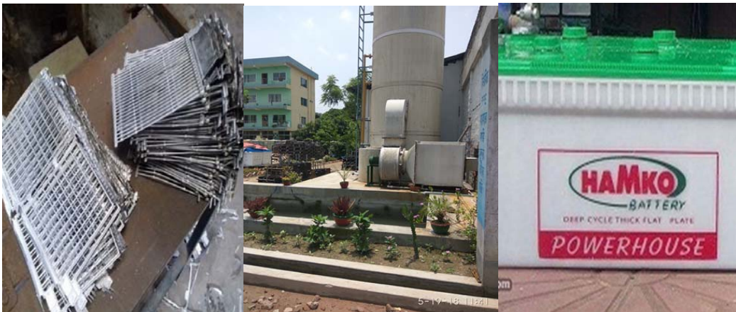
Figure 7 Lead Plate(Grid Shape)
