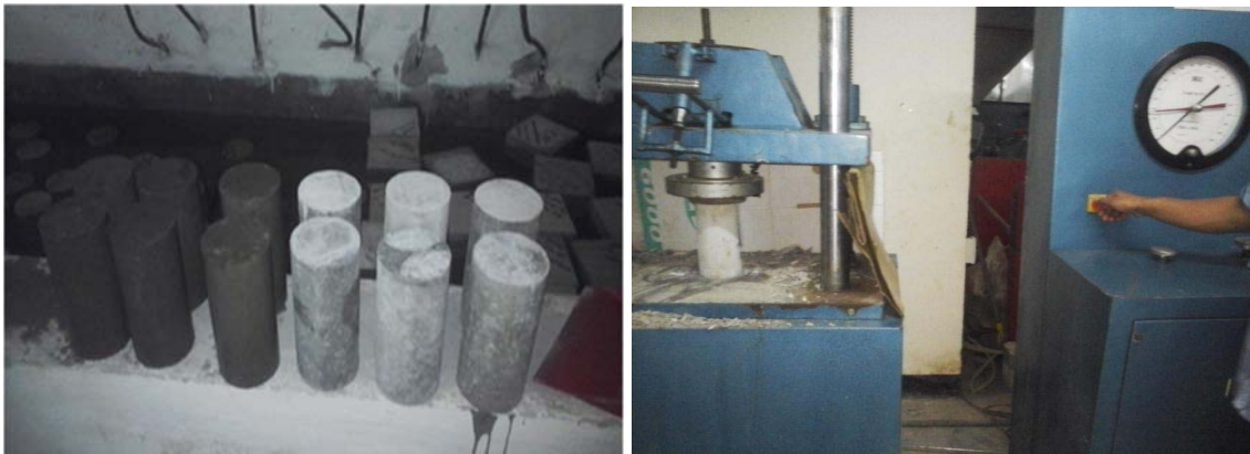
Figure 1: (a) Casted Cylindrical concrete specimen (b) Compressive Strength Test of Concrete
