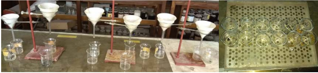
Figure 7: Sample preparation for suspended solids and total dissolved solids.
