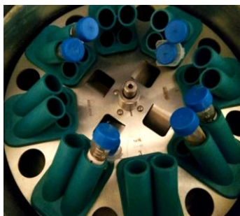
Fig.4 Centrifugation of decanted liquid
