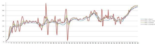
Fig.5 Sensor Data(RG) and Filter Data(B)
