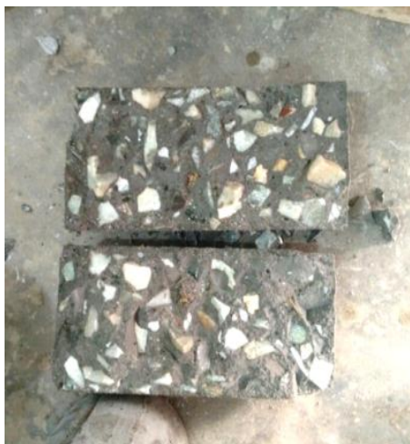
Fig.5 After tensile strength test
