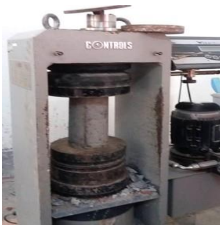
Fig.1 Equipment set-up of compressive strength test.
