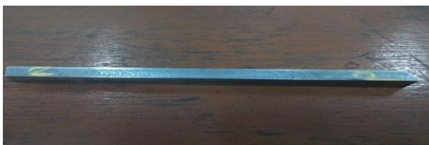
Fig.3 Prepared Work-piece after grinding, surface finishing and milling.
