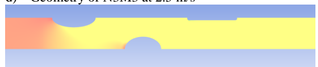
Fig 18: Pressure contour for water-vapor a) N6B1 at 0.5 m/s b) N6B1 at 2.5 m/s c) N3M3 at 0.5 m/s d) N3M3 at 2.5 m/s
