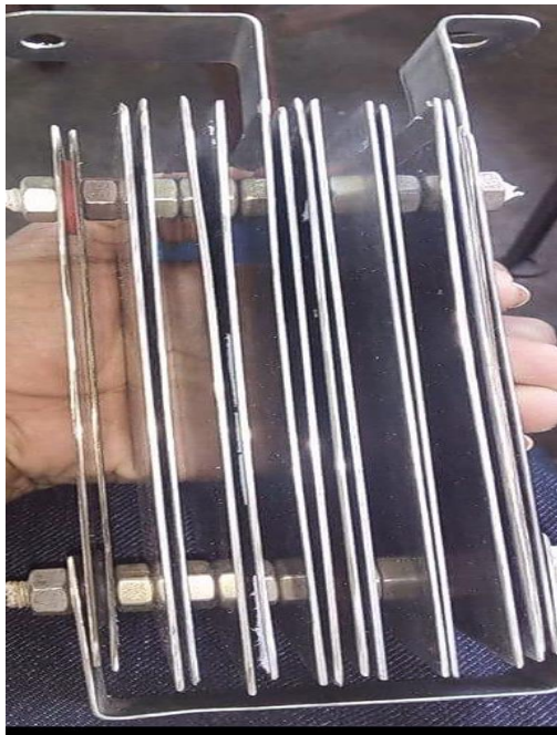
Fig 2 : 6 Plate HHO Cell
