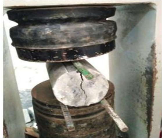
Fig.2 Equipment set-up of splitting tensile strength test
