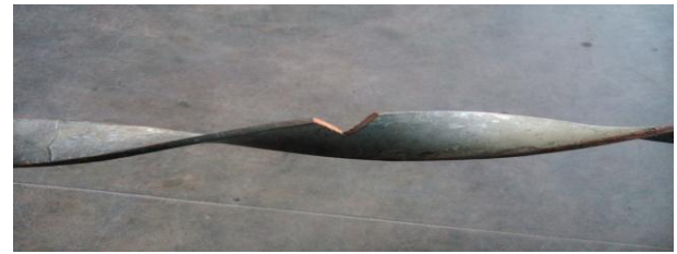
Fig. 3: V-shaped twisted tape insert of copper
