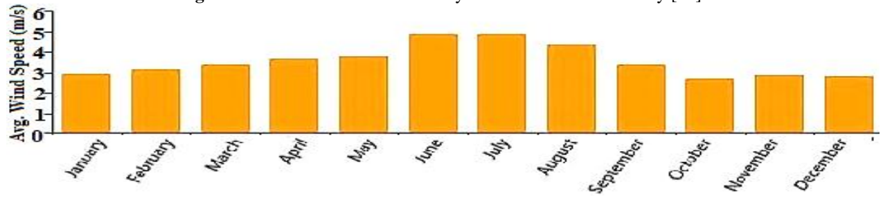
Fig.2 Monthly average wind speed data (NASA Surface meteorology and solar energy database).
