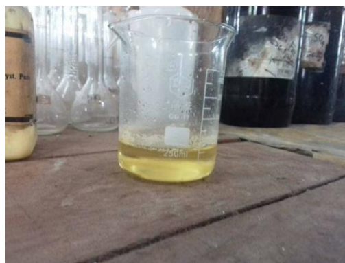
Fig. 4 Extracted biodiesel after separation
