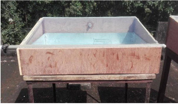
Fig.3 Fabricated single basin solar still
