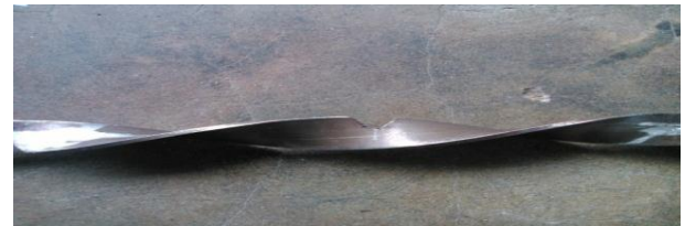
Fig. 4: V-shaped twisted tape insert of stainless steel
