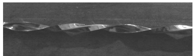
Fig. 2.1: Twisted stainless steel angle insert
