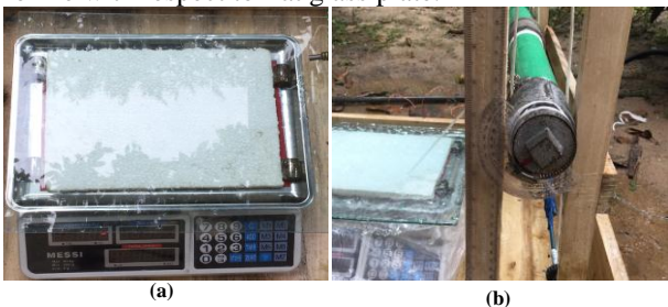
Fig. 3 (a) Weight measuring device with glass plate and roller; (b) Angular and vertical position measurement
