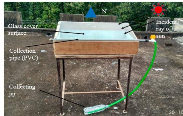
Fig.2 The fabricated conventional single slope single basin solar still.
