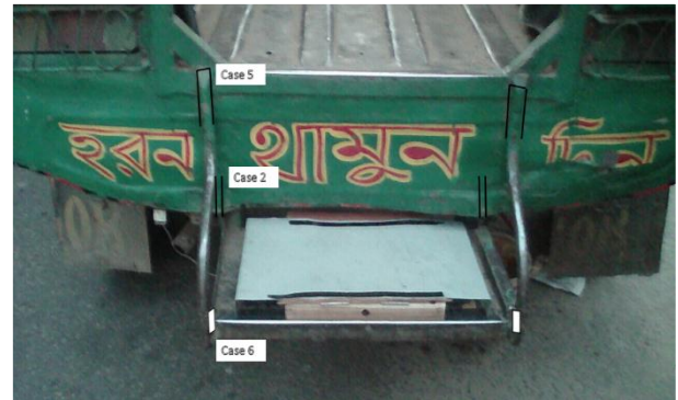
Fig.8 Analysis of footrest structure welded joint (All the cases are previously mentioned at Table 1.2)
