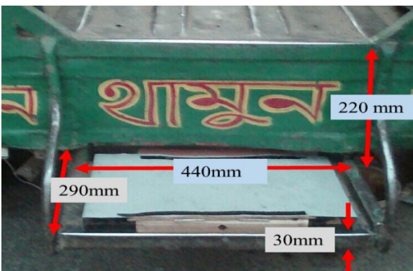
Fig.7 Necessary geometrical measurements of selected footrests
