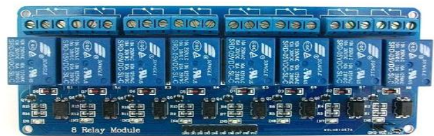
Fig. 10 Relay interface board
