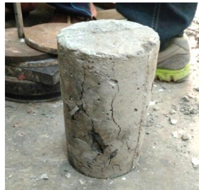
Fig.3 After compressive strength test
