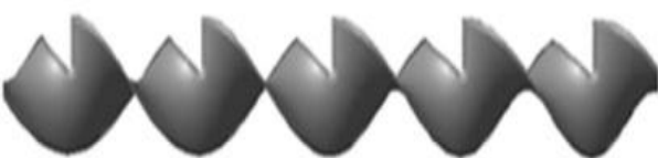
Fig. 2: Twisted tape insert with V-cut
