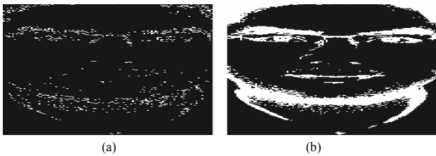
Fig. 7. Experimental example of the Labeling Image: (a) Canny edge image and (b) extracted labels in image.
