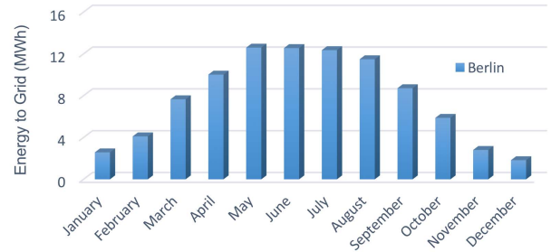
Fig. 5. Available energy to grid produced by the same 100 kWp system installed in Berlin.
