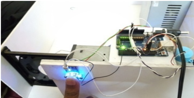
Fig. 5: Prototype of the system, finger placed on finger print scanner.
