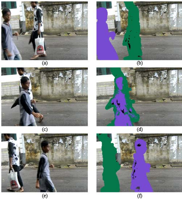
Fig. 3. Processing example of occlusion handling. Left and right column represents input frame and labeled frame respectively. (a) & (b) before occlusion, (c) & (d) during occlusion and (e) & (f) after occlusion.
