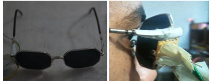
Fig. 7. Eye blink sensor design with correct angle (left) and placement of sensor to driver (right)
