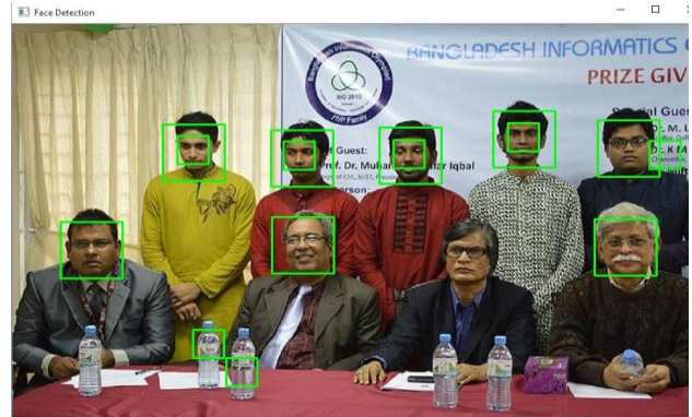
Fig. 2. PFS front ends for auto-annotation. The initial result detected by AdaBoost Algorithm.
