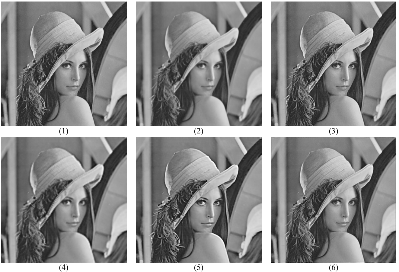
Fig. 4 Failed restoration case for previous method: (1) Original image, (2) degraded image, (3) restored with proposed method, (4) failed restored with previous method, (5) restored with [13], (6) restored with Matlab's deconvblind.
