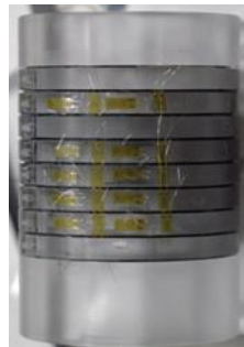
Fig. 2 Installation of strain gauge
