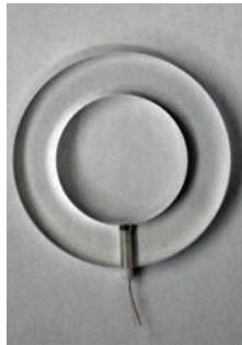
Fig. 1 Installation of small-sized water pressure gauge
