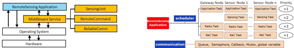
Fig. 7. Outline of the RemoteSensing application structure and its implementation in FreeRTOS [8].
