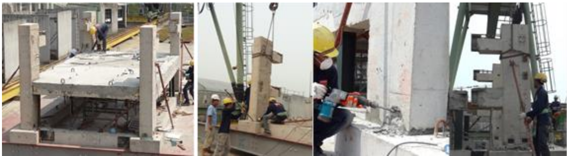
Fig. 10. Half-scale models of DfD prototypes
