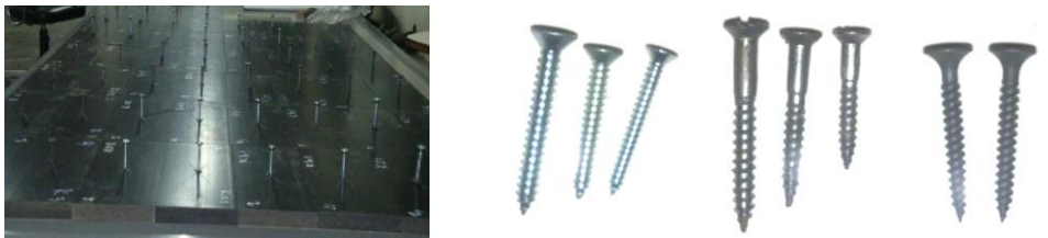
Fig. 12. (a) Specimens for Withdrawal Test; (b) Sheet metal, cut thread wood, and fine thread drywall screw
