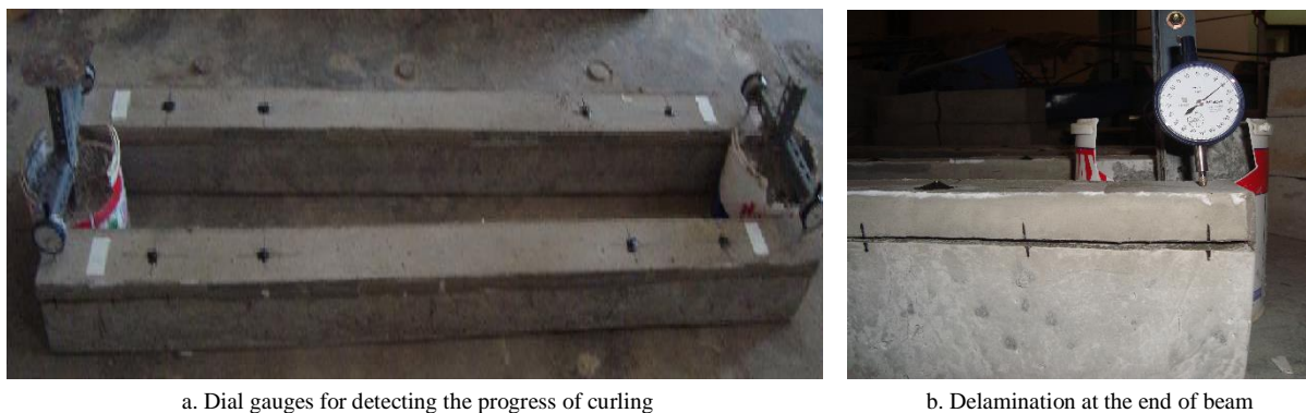
Fig. 3. Measurement of delamination tendency
