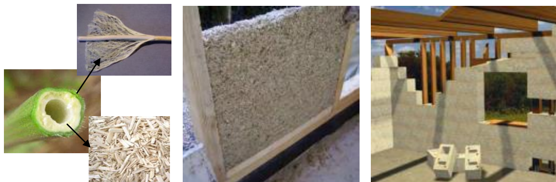
Fig. 1. Hemp concrete and practical application in wall building, redrawn with photo from ref. [11].
