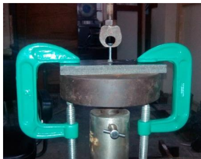
Fig. 13. Schematic of Screw Withdrawal Test
