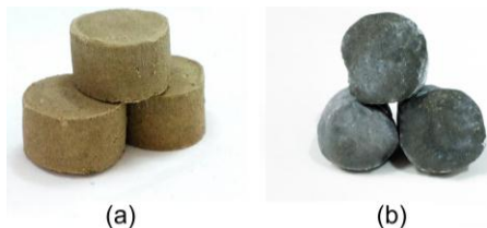
Fig. 1. (a) diatomite pellet capsule (b) coated capsule with cement paste ( w/c=0.5 )
