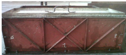
Fig. 1. Steel mold for casting specimen made of steel plate of 6 mm thick.
