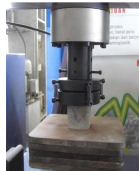
b. Compressive strength test
