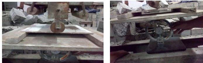
Fig. 2. Flexural strength test with proving ring machine
