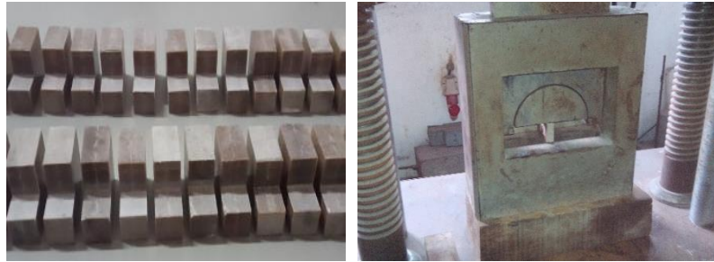
Fig. 8. (a) Specimens of Shear Test; (b) Shear Apparatus for Shear Test
