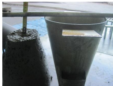
Fig. 10. Slump test of the mix with 100% of recycled sand at 90 minutes. The slump-flow test was unfeasible even though at 15 min it was a SCC with a spread of 680 mm
