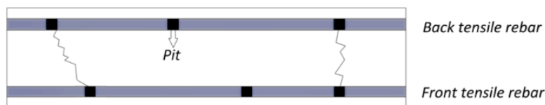
Fig. 1. Plan view of potential pit locations and possible interference of localized corrosion between adjacent tensile rebars [15].
