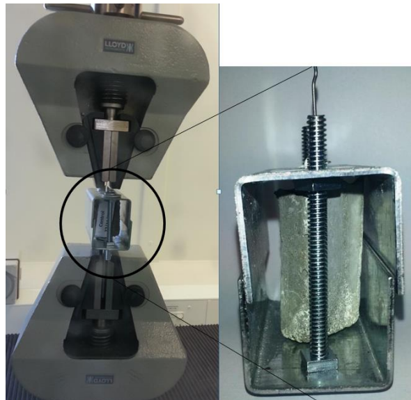
Figure 2-Apparatus of pull-out test
