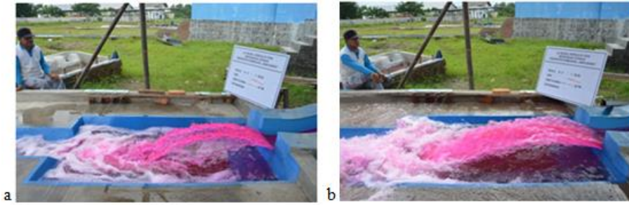
Fig. 6. Water jump condition in plunge-pool, model series-0: (a) Q_{1000} , (b) Q_{PMF}
