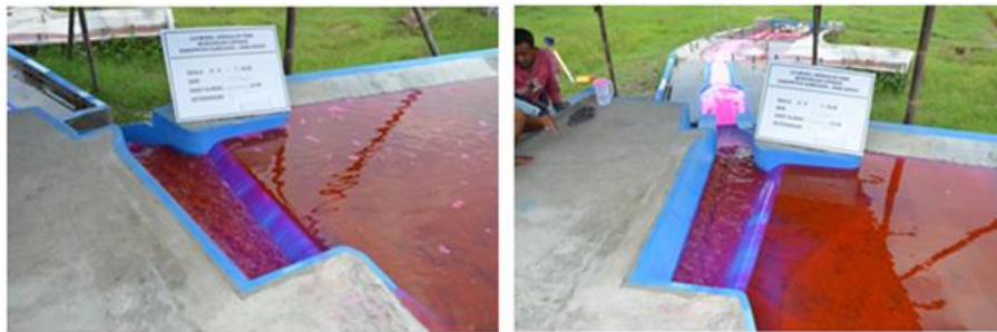
Fig. 9. Flow condition on side-channel and chuteway, Model Series-2 Q_{1000} .
