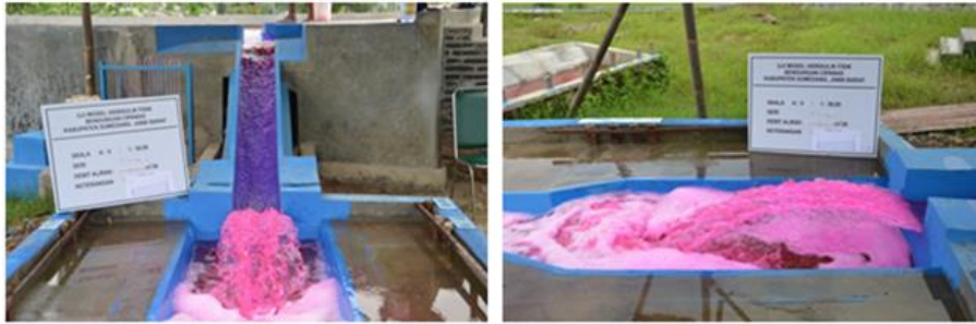
Fig. 10. Water jump on plunge-pool, Model Series-3, Q_{1000}
