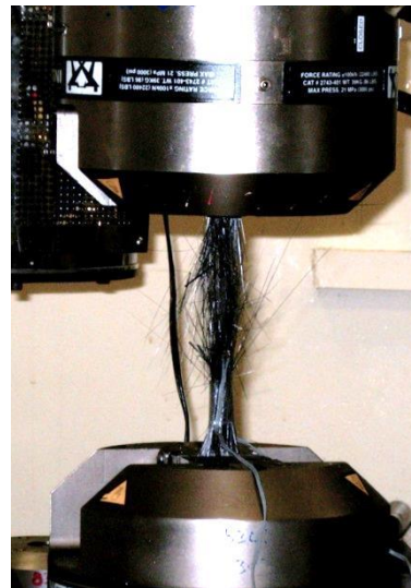
(c) Sample after breaking.
