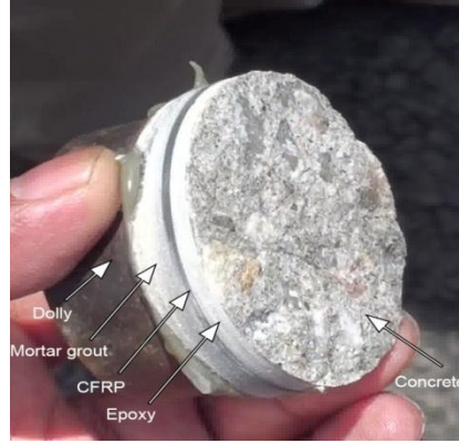
(b) Pulled off dolly showing failure in concrete.
