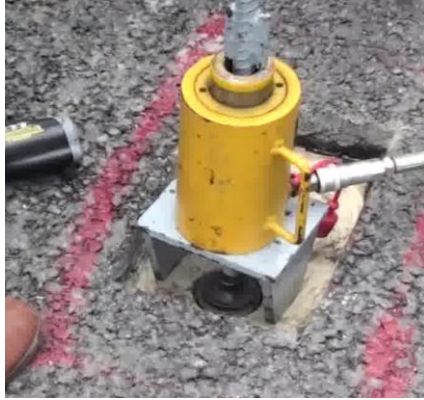
(a) Dolly subjected to pull-off force by hydraulic jack.
