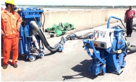
(a) The blast cleaner machine
