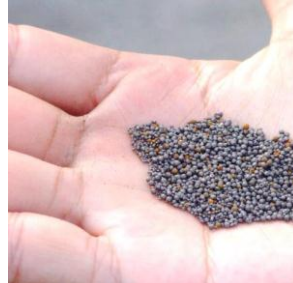
(b) Steel shots used in blast cleaning
