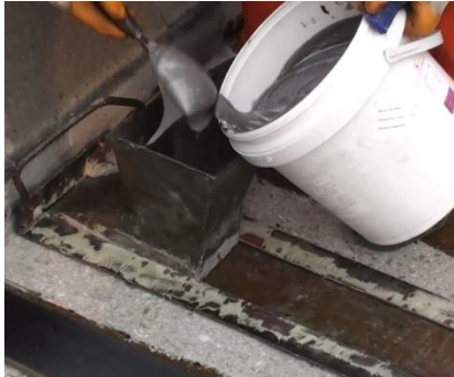
(a) Putting epoxy glue in the sliding hand mould.
