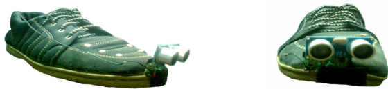
Fig 5: RF transmitter part (placed in a shoe) of our Solar-powered digital hat
