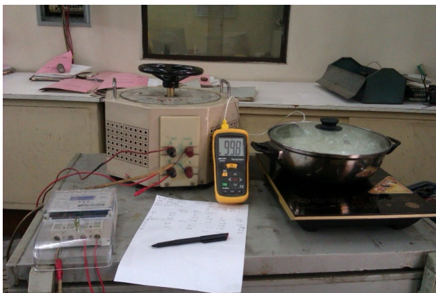
Fig. 6 Experimental set up for cooking using Induction cooker
