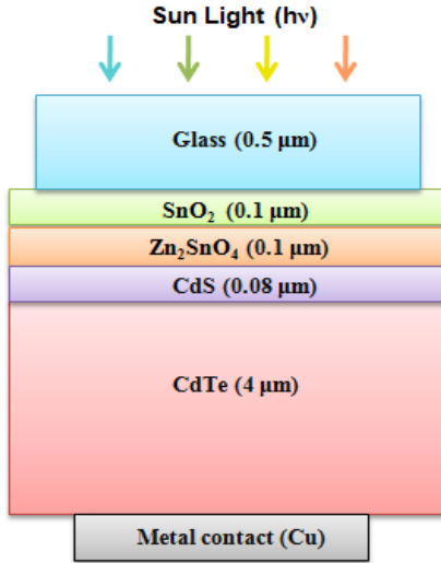
Fig.1 The conventional CdTe solar cell structure
