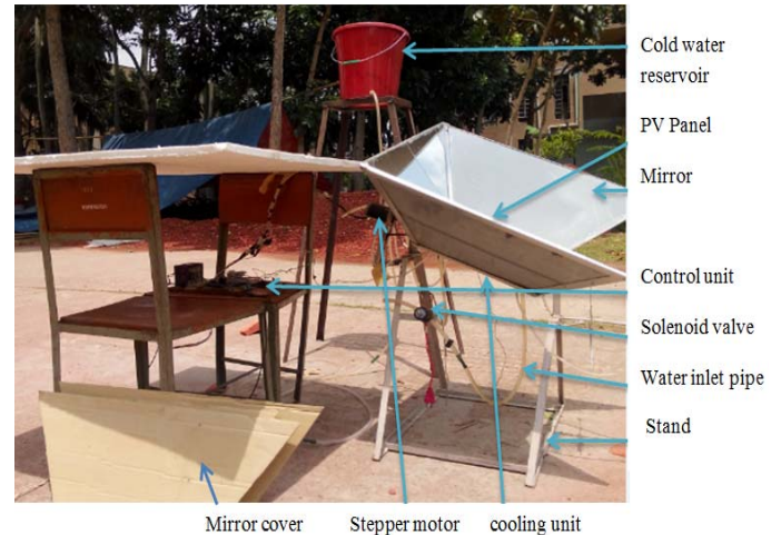
Fig. 4 Constructed mirror reflected solar panel
