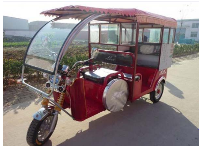
Fig. 1. A typical easy bike for five passengers in Bangladesh
