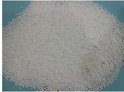
Fig. 4 Polystyrene micro beads used as insulating material in the cooker
