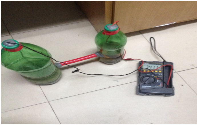
Fig. 3. Practical setup of MFC system shown in figure 2
