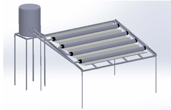
Fig. 1: Schematic of Proposed Evacuated tube solar collector
