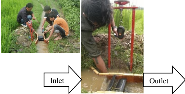
Fig. IV.3 Testing site (left) and torque measurement, head difference (right)
